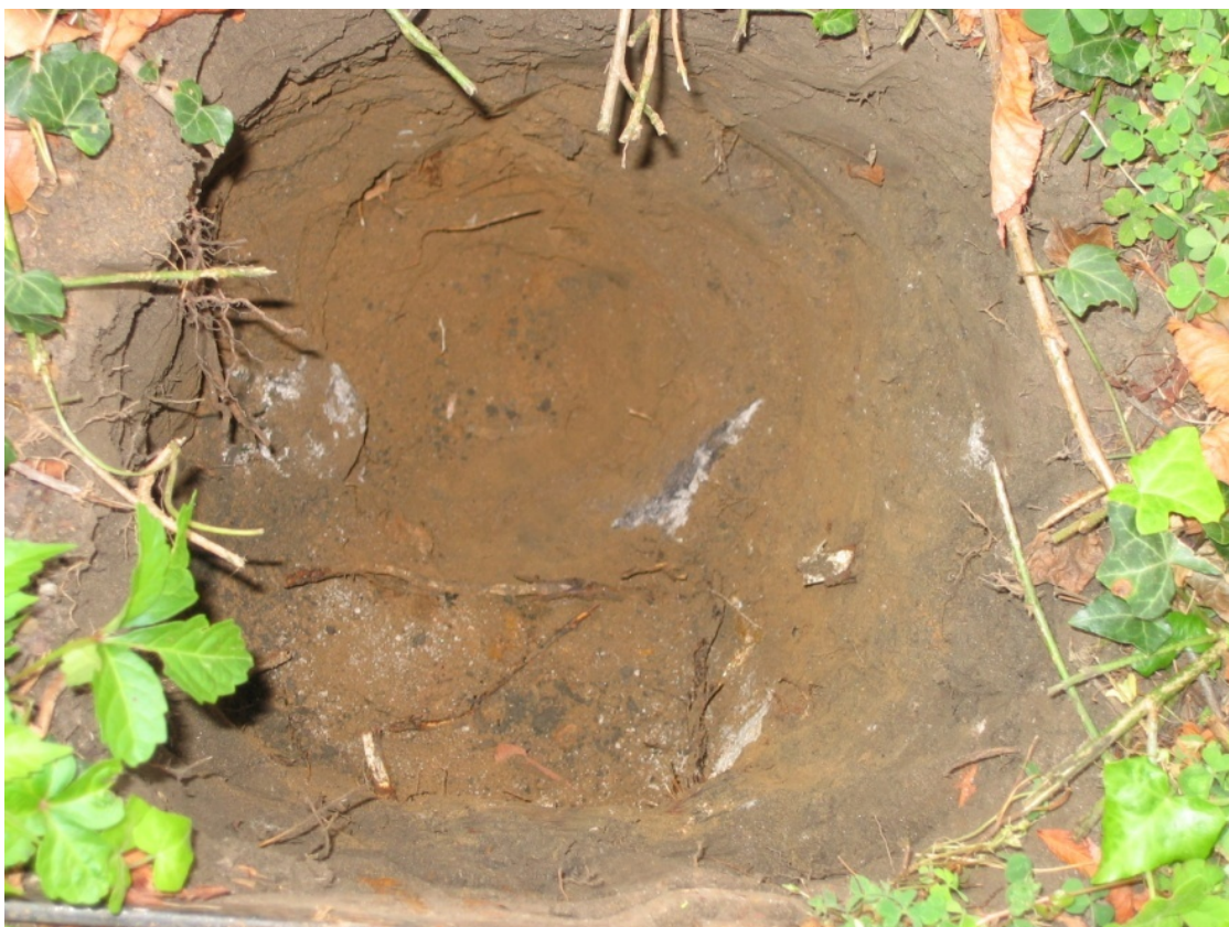
Figure 15: Typical soil stratum within the Postholes
