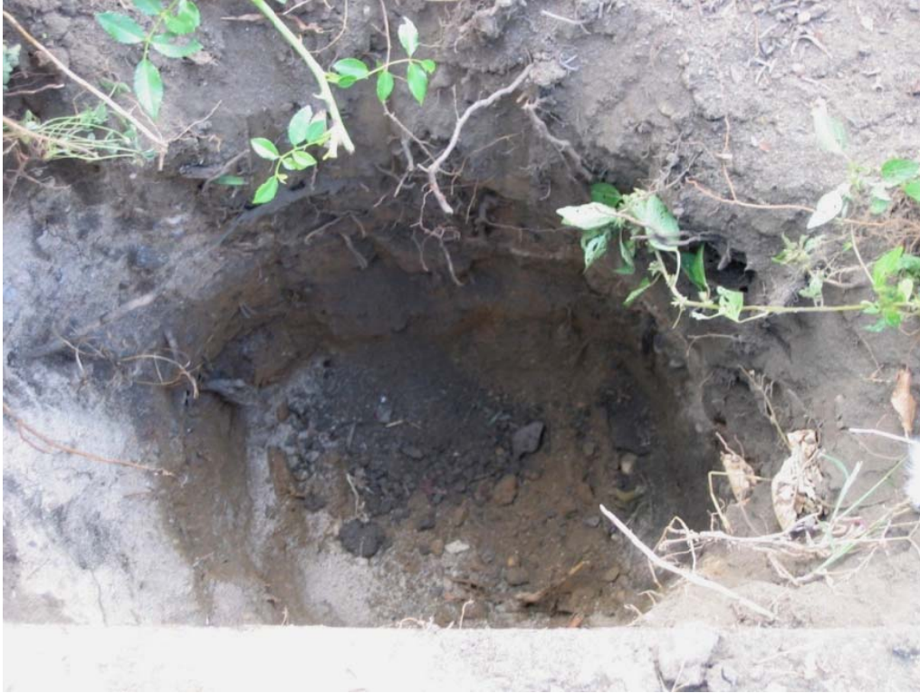
Figure 16: Typical soil stratum within the Postholes
