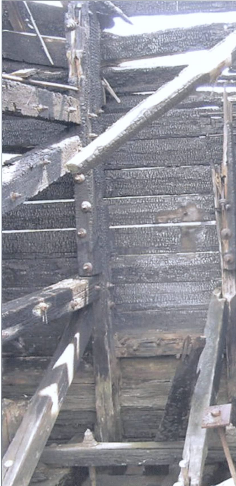
Figure 5-95. Detail showing outer wing frame. Note second futtock location. View to the east (starboard).
