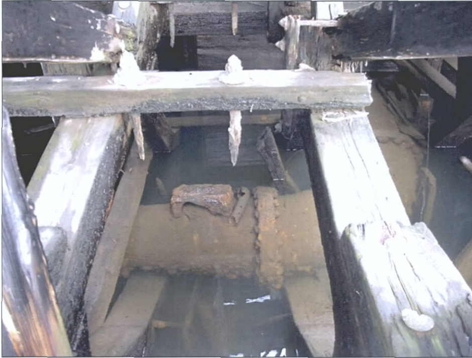
Figure 5-156. Outlet pipe. Outlet in upper right of image corresponds with the outer hull fitting in Figure 5-148. Port wing, view to the west (port).
