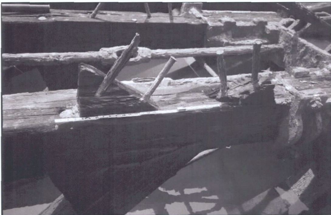
Figure 5-106. Detail of main deck beam showing truss chocks and fasteners. Starboard wing, view to the south (aft).
