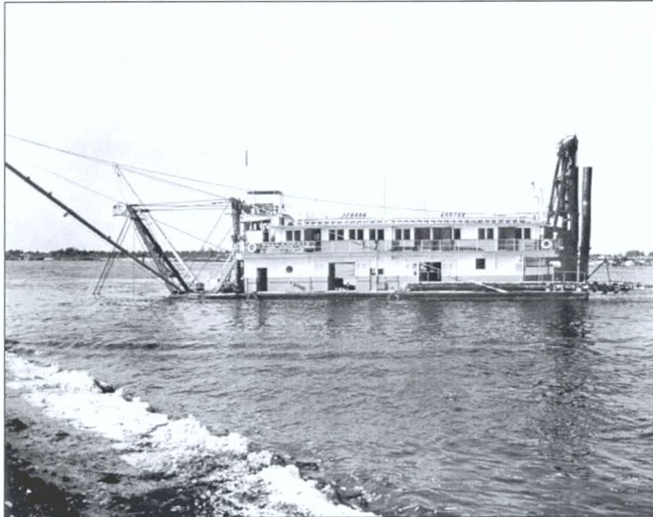
Figure 4-16. Cutterhead dredge Hallandale , similar in form and size to V36, at work in the Intracoastal Waterway, Fort Lauderdale, Florida, circa 1954. Note A-frame at bow and spuds at stern (photo courtesy of the Florida Photographic Collection).
