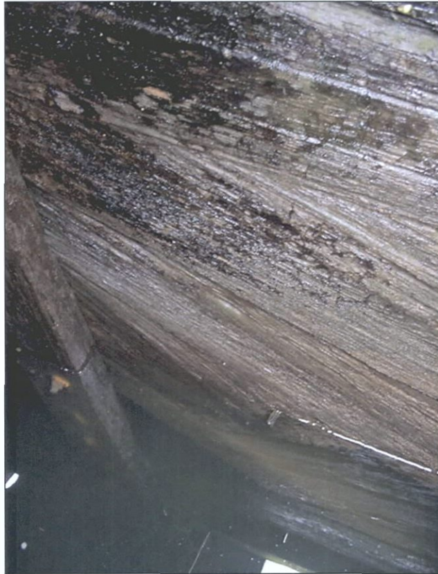
Figure 5-59. Confluence of trusses at centerline bulkhead (T1). View from port toward centerline, to the southeast.
