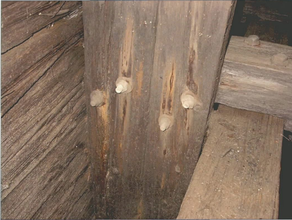
Figure 5-55. Side frame detail. Note edge fastened futtocks, deck beam, and longitudinal stringer under deck beam. Outer hull planking is left. View to the north (forward).
