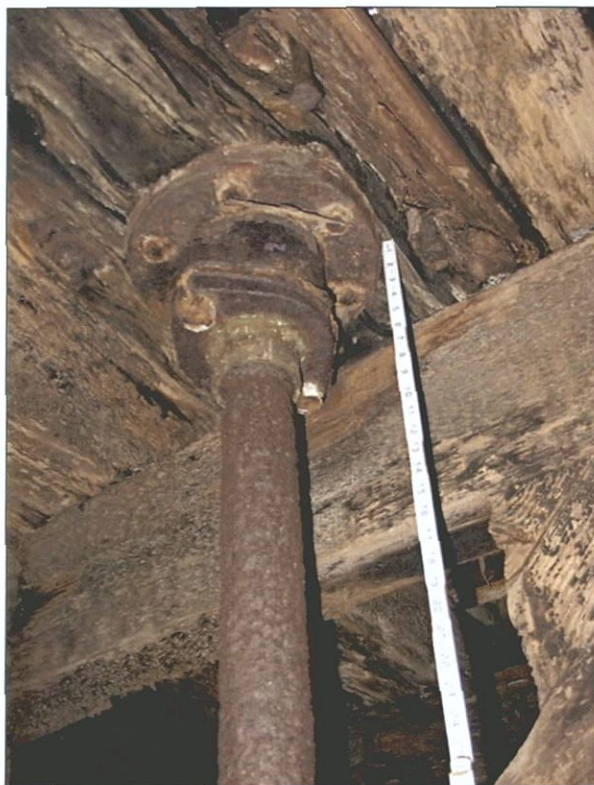
Figure 5-155. Impeller driveshaft pass-through fitting in upper wing deck.
