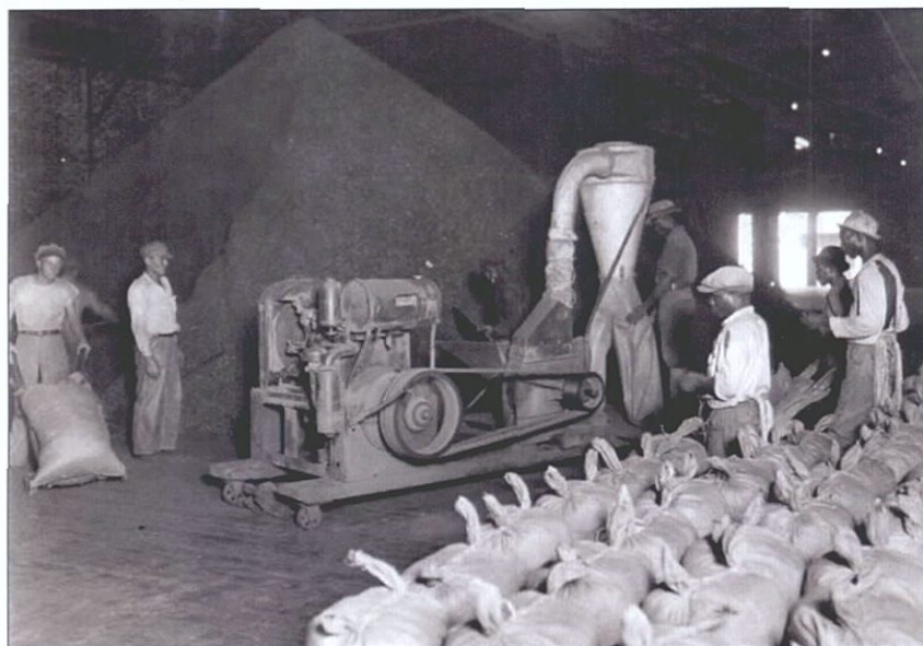
Figure 7-22. Dried scrap bagging operation (photo courtesy of State Historical Society, Wisconsin).
