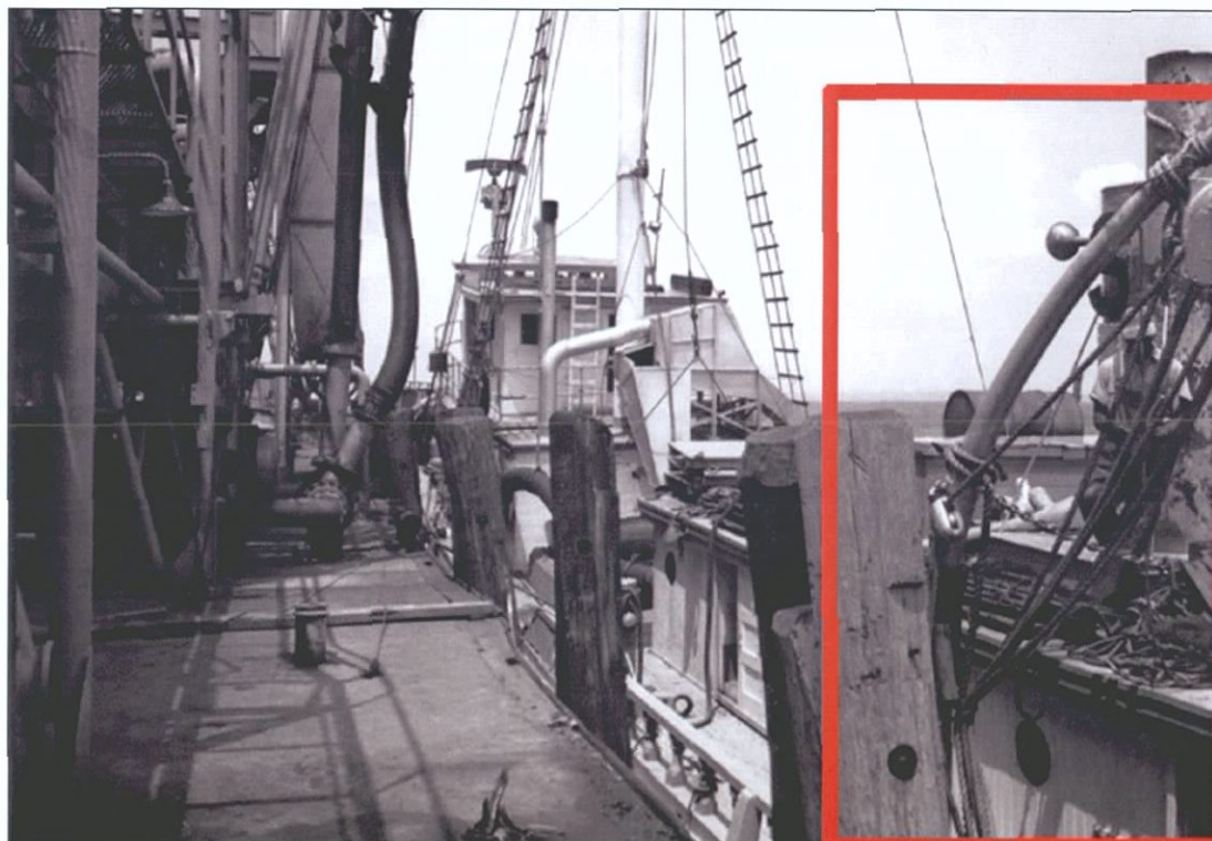
Figure 7-98. Port side of Mermentau , showing forward davit.
