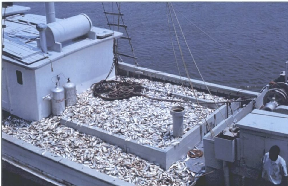
Figure 7-93. Historical photo of a menhaden vessel, showing standpipe in similar location to Fish Hawk (photo courtesy of NOAA).
