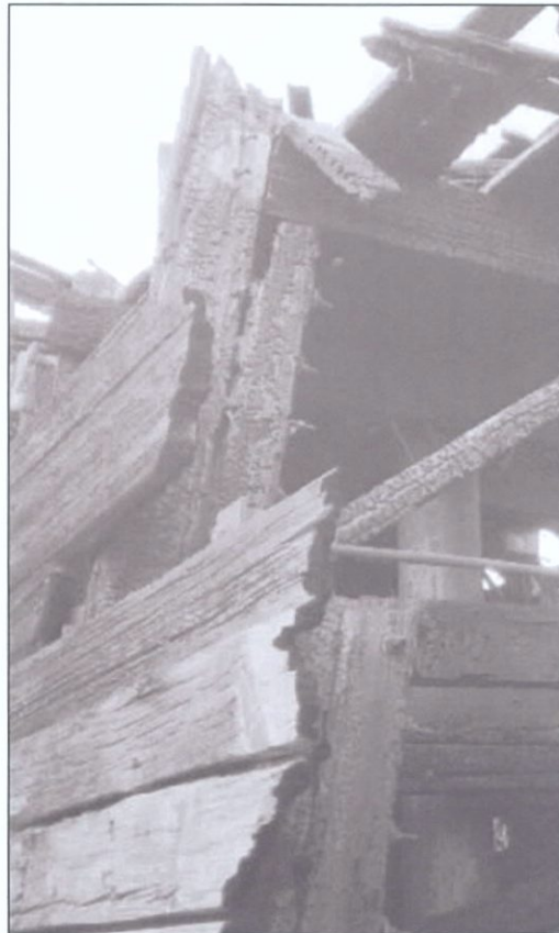
Figure 5-99. Inner wing frame. Note upper deck at top of photo, also seen in Figure 5-96. Starboard wing view to the north (forward).
