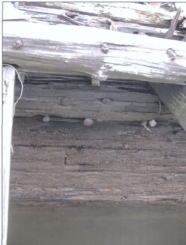
Figure 6-82. Starboard side looking starboard (east) showing extant mold ceiling. Note composite shelf just below deck beams.
