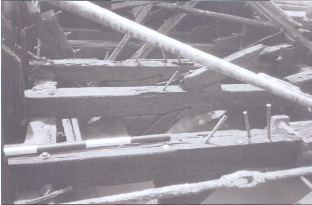
Figure 5-63. Exposed northern end of V1, showing Truss 8 and main deck beam. Note truss attachment under deck beam at center of photo. Also note use of triangular chock. View to the south (aft).
