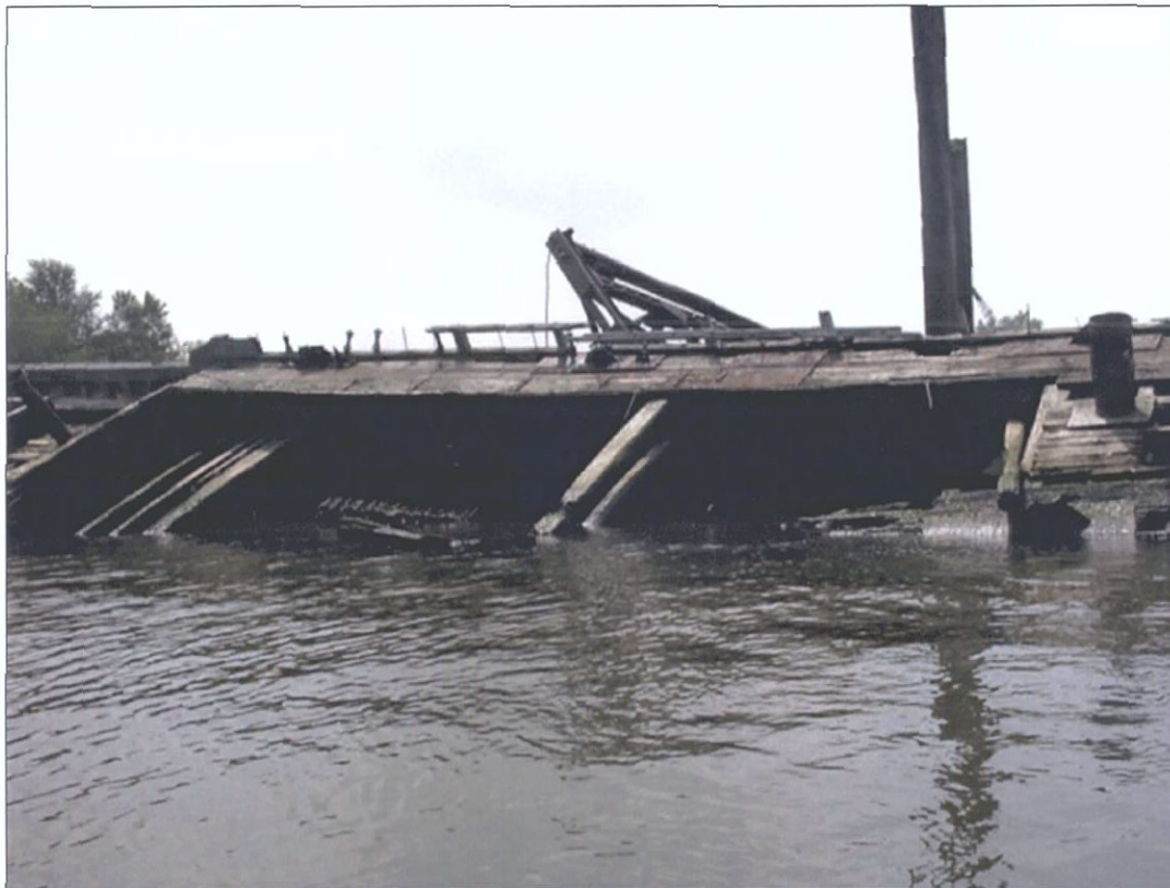
Figure 7-96. Starboard quarterdeck, looking west. Note from left to right: bollard, forward davit, large plate, aft davit, and aft stack. Also note small steel deck plates adjacent to aft deckhouse.
