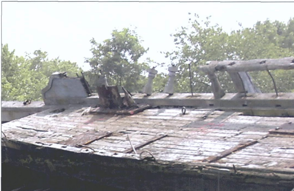
Figure 7-79. Starboard side of vessel showing rail with decorative stiles. View to the southwest.
