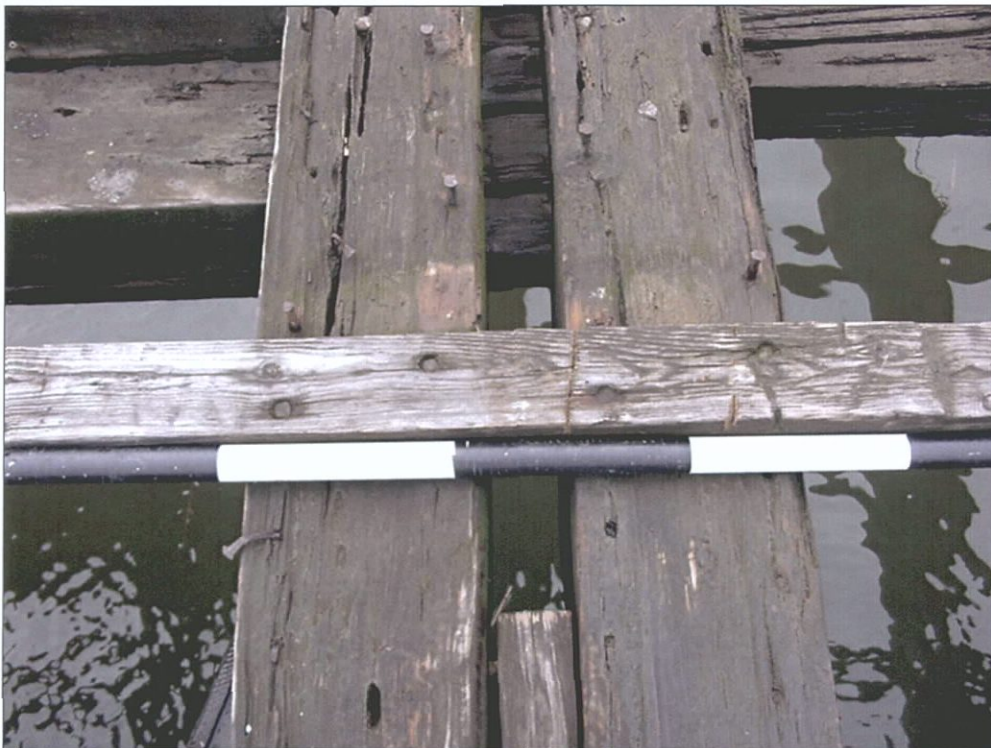
Figure 6-83. Single remaining deck plank just starboard of forward hatch. Note rose head spikes and fastener pattern.
