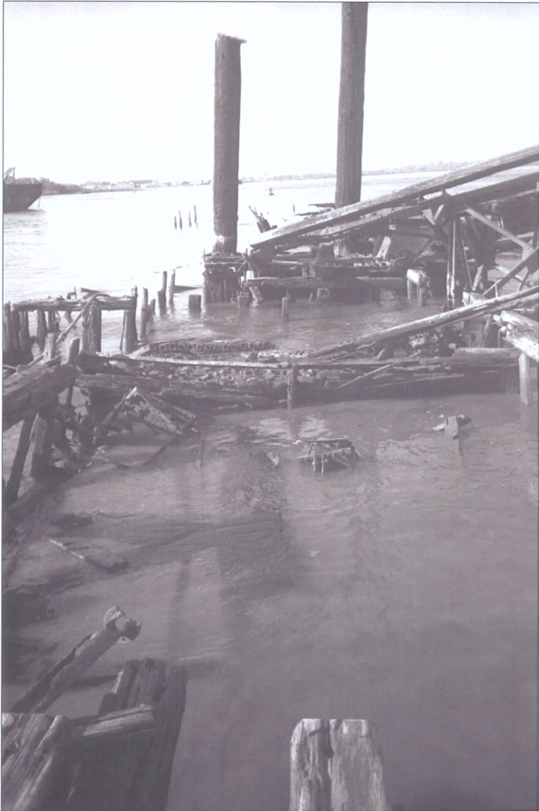
Figure 4-25. V36, general view of the main deck. View to the north (aft). Note spuds and collapsed A-frame.
