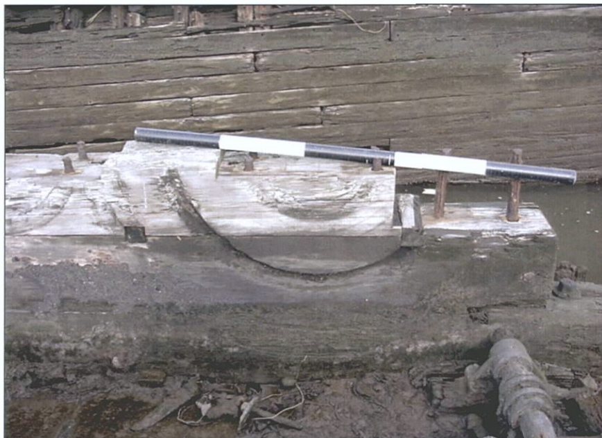
Figure 4-54. Close-up of port side cable mount, showing circular wear from cable spool. View to the east (port).
