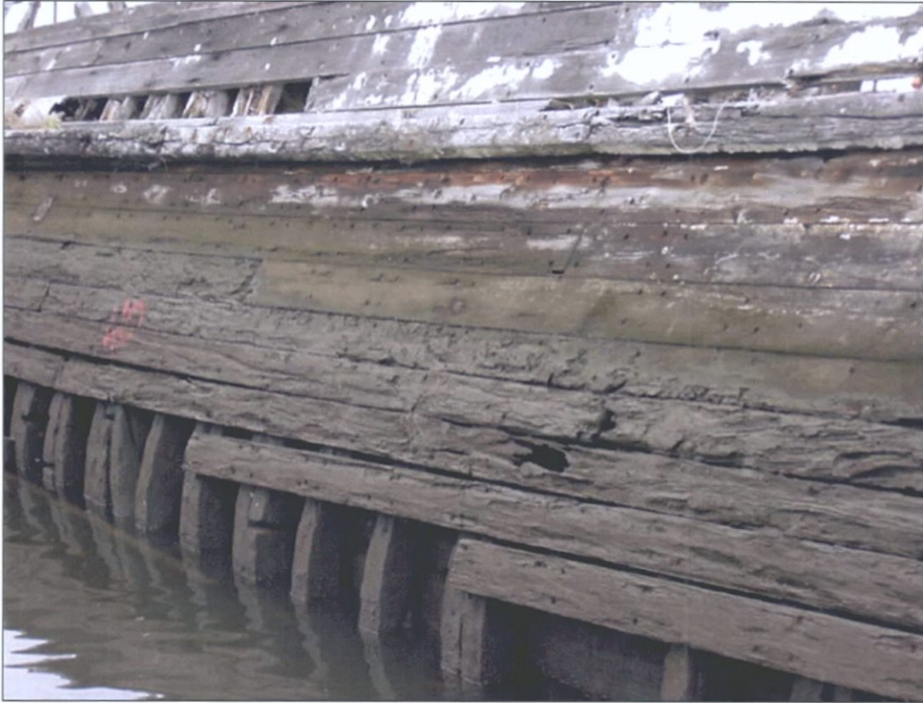
Figure 7-49. Starboard side view, looking northeast, of midship section showing exposed framing at the turn of the bilge.
