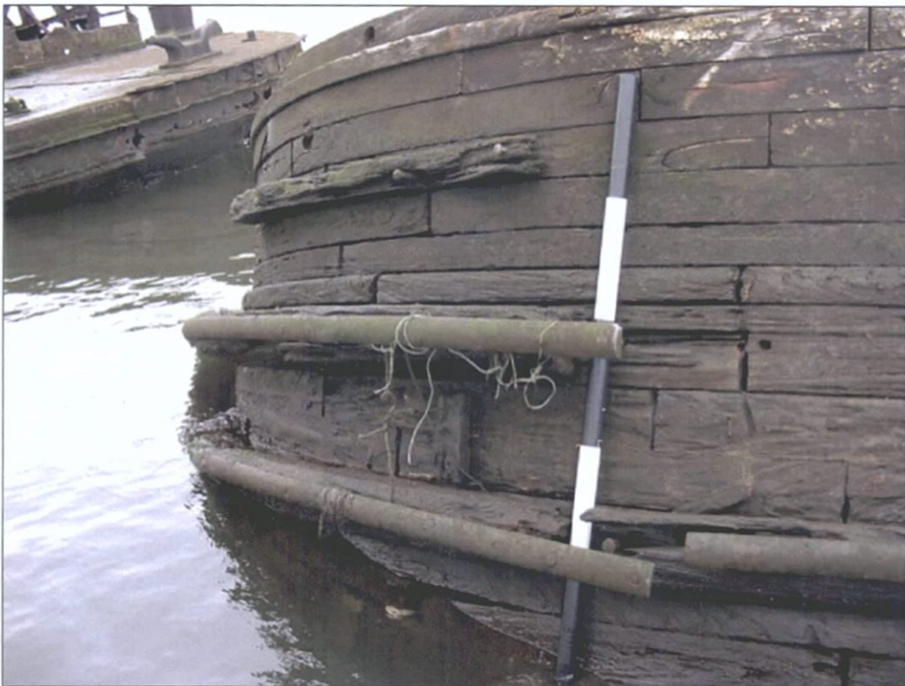
Figure 7-47. Close-up of fantail assembly. Note short timbers and rub rails. View from starboard looking east.
