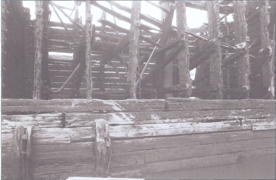
Figure 5-32. Close-up of starboard side, view to the southwest. Note outer hull planking with butt joints.
