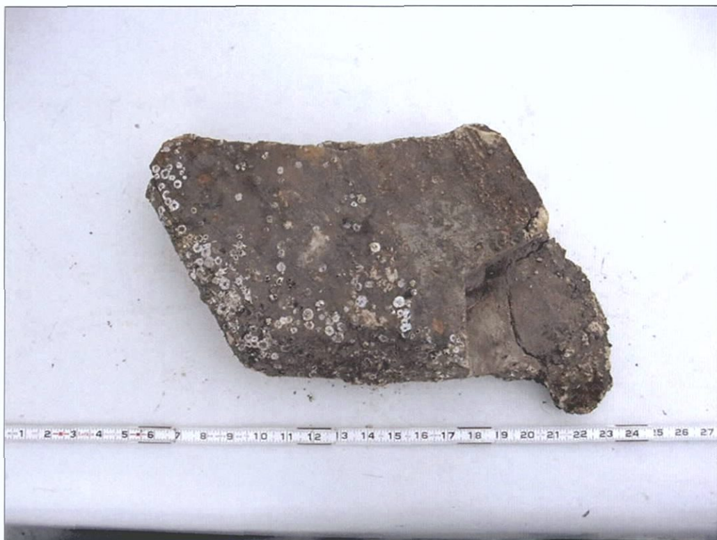
Figure 8-31. Section of concrete boiler bed.
