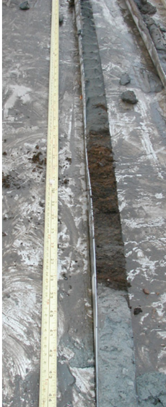
Figure 7. GP27 showing the sequence of very dark gray (N3) silty lacustrine sediments, very dark brown (7.5YR 3/3) organic tidal marsh surface, and gray (2.5Y 6/1) sandy fluvial/estuarine sediments. Note: tape shows scale not depth. Brooklyn Navy Yard, Kings County, New York (PCI 2009).
