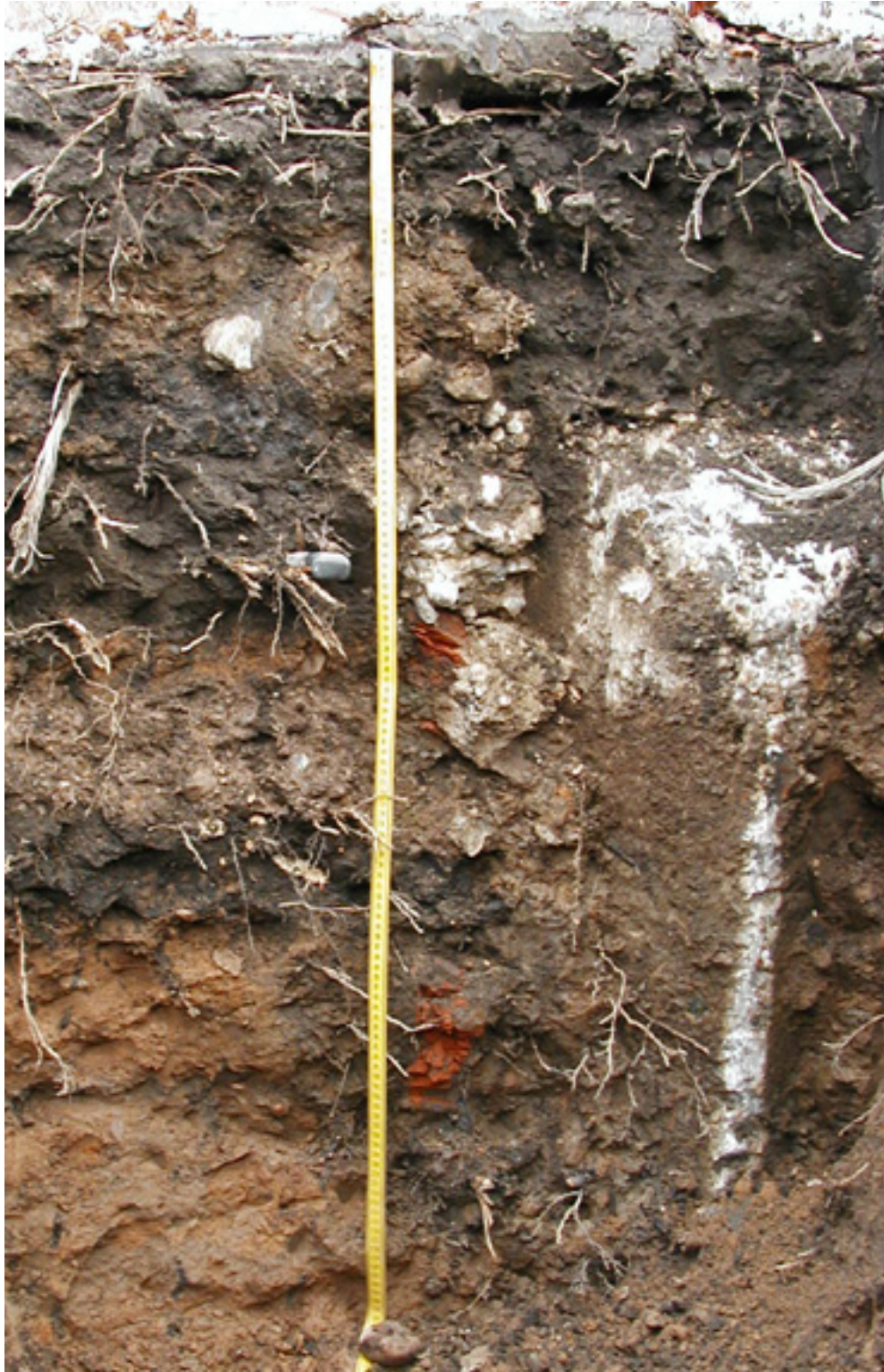
Figure 9. Profile from T2 showing stratified historic fill. A concrete pillar extending beyond the bottom of the trench is in the right side of the profile. Brooklyn Navy Yard, Kings County, New York (PCI 2009).
