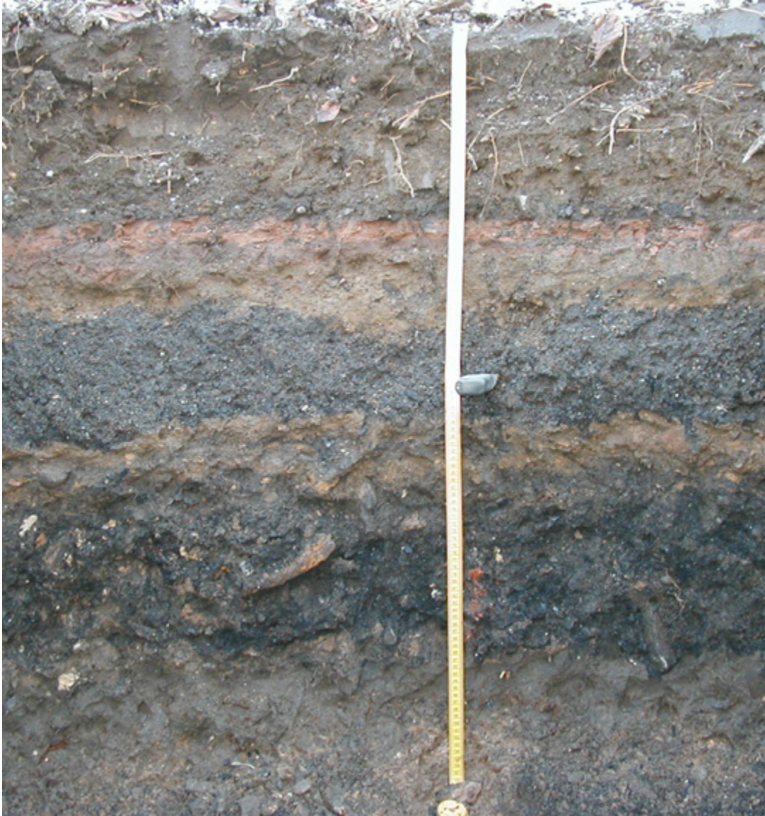
Figure 8. Profile from T7 showing stratified historic fill. Soil knife at 50 cm is in a layer of ash and slag. A second layer of ash and slag from 70 to 96 cm has brick and iron. Brooklyn Navy Yard, Kings County, New York (PCI 2009).
