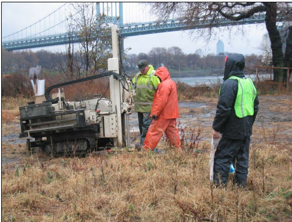
Figure 2. Example of the larger track-driven geoprobe.
