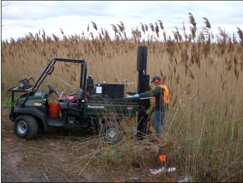
Figure 1. Example of smaller geoprobe mounted on a wheeled mule.
