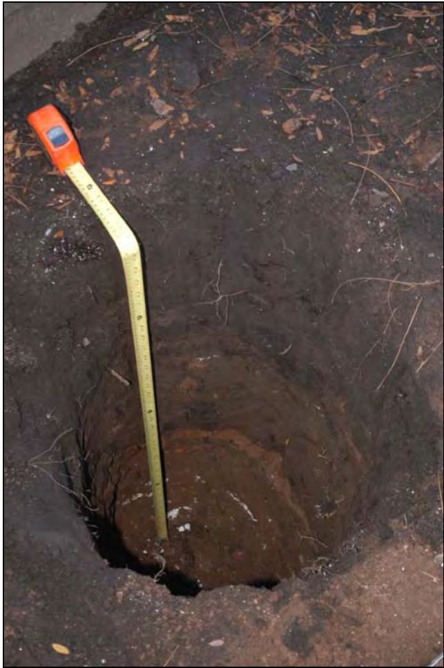
Photo 2 - Profile of Test #1 at Trinity Church. Note the ight Sand Layer underlain by Shell and Brick.
