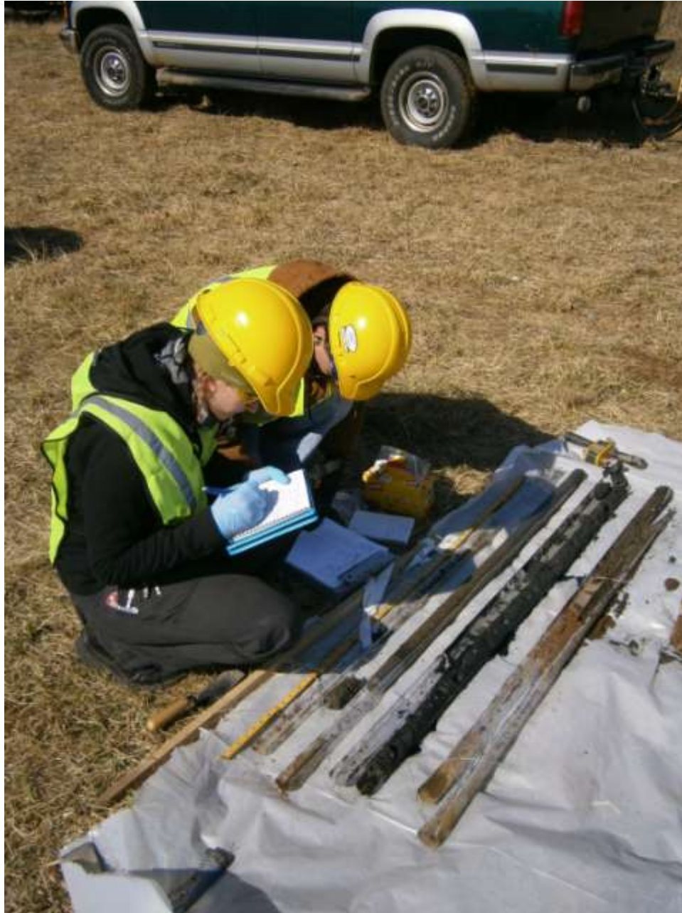
Figure 5. Split cores documented and sampled in the field by GRA field staff.
