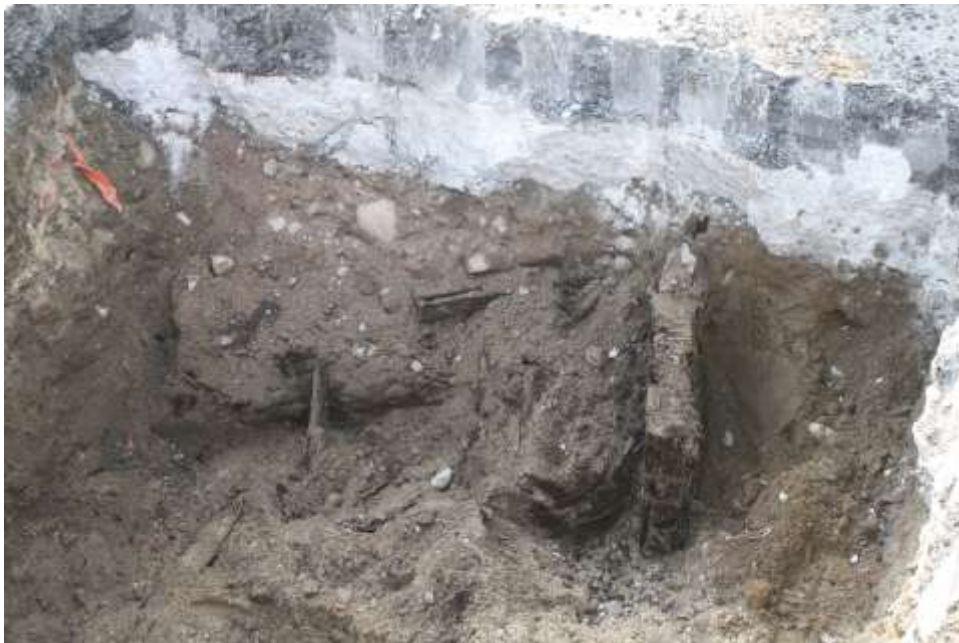
Image 73. OF/Water, wood in E wall of test pit
