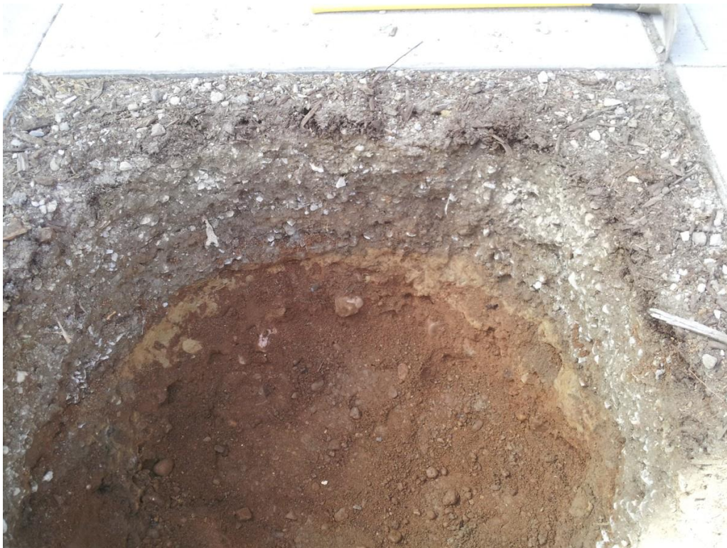
Photograph 51: (4/12/12 memo) East 127 th Street, south side, Pit 4, looking south, showing sub base over a layer of dark yellowish brown fine sandy fill over a brown fine sandy fill level.
