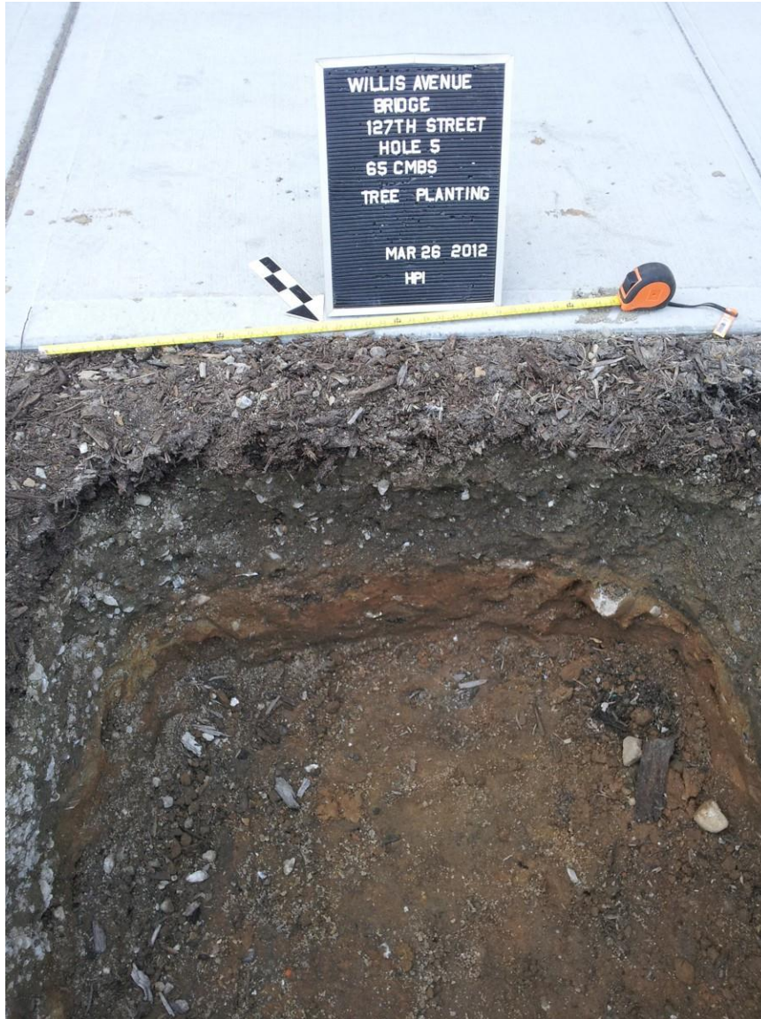
Photograph 52: (4/12/12 memo) East 127 th Street, south side, Pit 5, looking south, showing sidewalk sub base over brown silty sandy fill. The measuring tape is set at one meter (3.3ft) in length.
