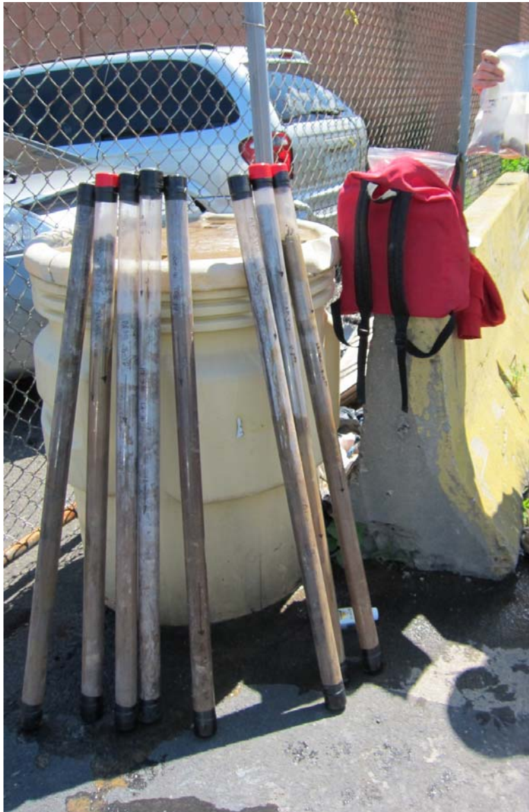
Photo 4 View of eight four-foot-long geoprobe soil samples from AP-301 and AP-302, before transport to AECOM archaeology lab for processing and analysis.
