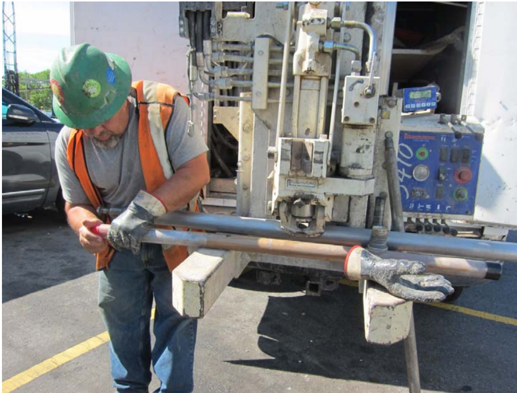
Photo 3 View of four-foot-long geoprobe soil sample encased in clear plastic being capped.
