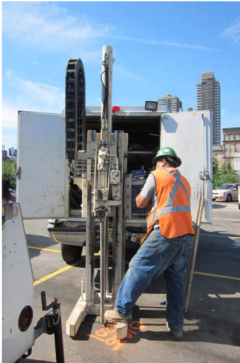
Photo 2 View of geoprobe rig in operation at AP-301, the former rear yard of historic Lot 11.
