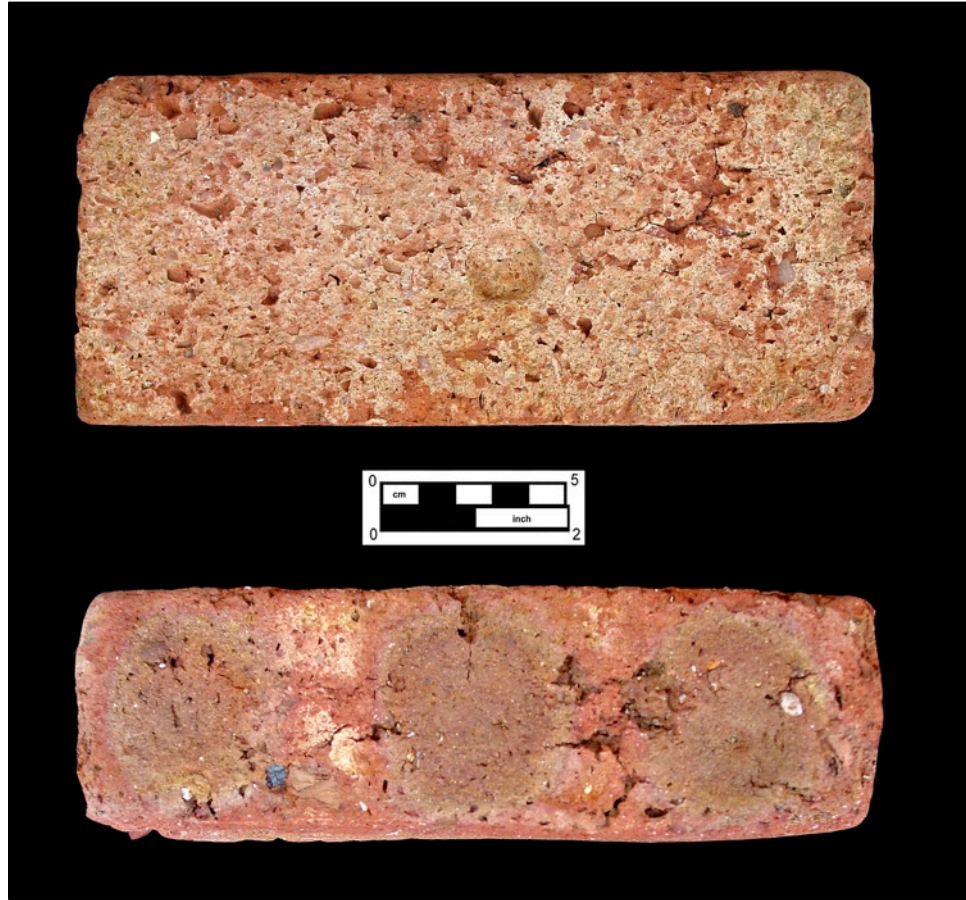
Image 8.14: Brick with “key” depression on the top and kiln scars on the side (FS 281.1). The other architectural artifacts consist of a rusted cut spike and a rusted screw, a few fragments of mortar ( n=3 ) and plaster ( n=1 ), a piece of cut wood, and a small piece of slate that is probably from a roofing tile, but might be from a slate writing board.
