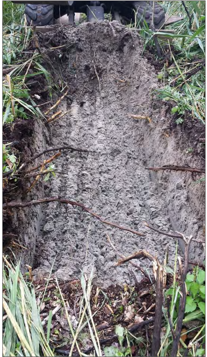
Light gray sandy soils observed throughout Trench 7, excavated near the northern boundary of the site
