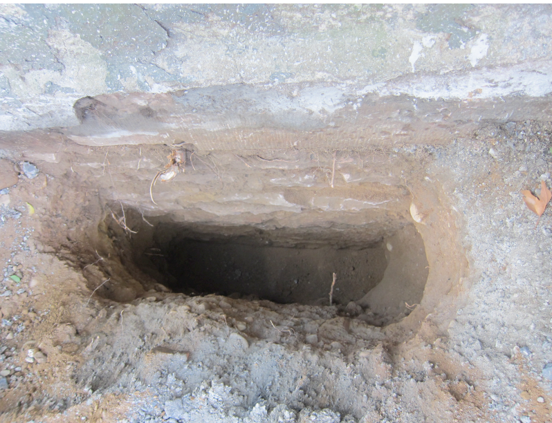
Photo 5. Looking into the test pit at the end of the excavation. Founding stones, which undoubtedly would be found below the wall, were not encountered in the 5-foot (1.5-m) deep excavation. (9-19-14)
