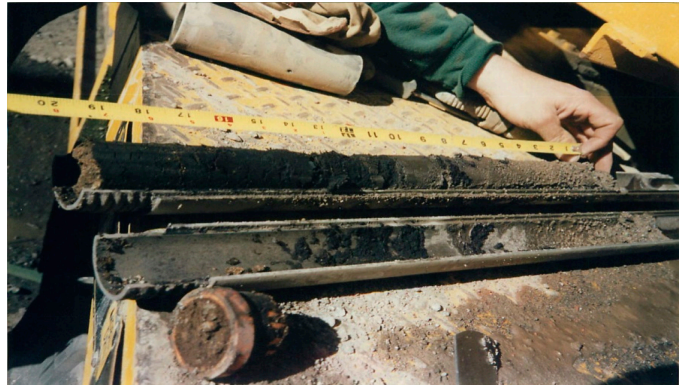
Figure 9. Deposit recovered from boring B1 at a depth of 24-26 feet (7.3-7.9 m) is being measured in the sampling spoon before transfer to glass collection jars. The lower part of the sample [left] is peat. (Geismar 4-14-99)
