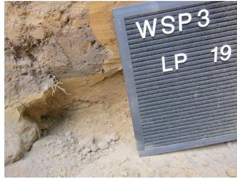
Photo 1. (above) East wall of LP19. The gray sand in the upper left corner is evidence of a previously backfilled utility trench. The “yellow” sand next to and below the trench is old park fill (an animal bone was found below the trench fill). See Figure 4e for a schematic profile. (Geismar 7-10-12)
