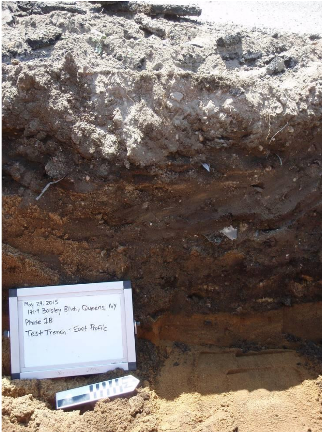
Photo 4: View of the eastern profile of the exploratory trench, facing west. Trench was excavated through blacktop and approximately 2.5 feet of cinder and asphalt rich fill. The base of the trench was a clean, culturally sterile sand layer (Stratum II). Photograph taken by K. French 5/29/15.
