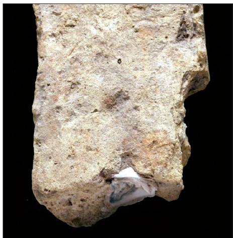
Figure 81. Broken yellow brick with a large piece of an oyster shell, probably accidentally included.
