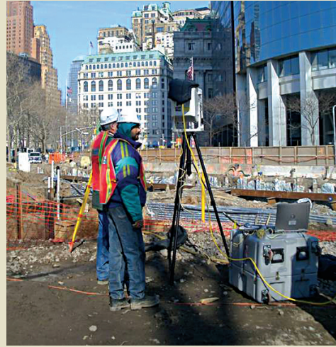
Figure 19. MTA specialists prepare their equipment to laser scan Wall 1.
