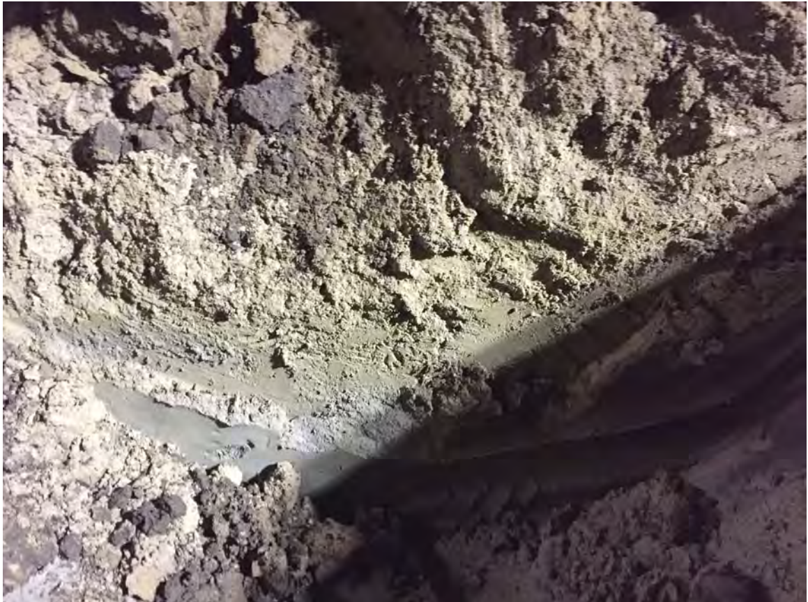
Plate 13. Profile of sediment near EP-102, reaching a depth of approximately fourteen feet below ground surface (bgs). The sediment appears natural, with the historic water table boundary at about 12.5 feet bgs evidenced by gleying of the sediment.
