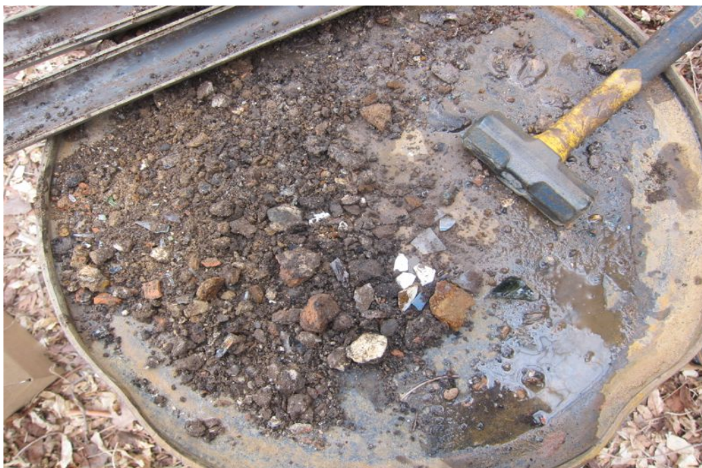
Photo 13. Sample of the fill in B2 recovered from a soil boring intended to determine the function of this circular feature originally identified as cistern. The depth of the fill, which proved to extend beyond 31 feet (9.5 m) below the feature surface, established that it was a well. The sampling spoon is in the upper left corner. (Photo: J. Geismar 4-8-2016)
