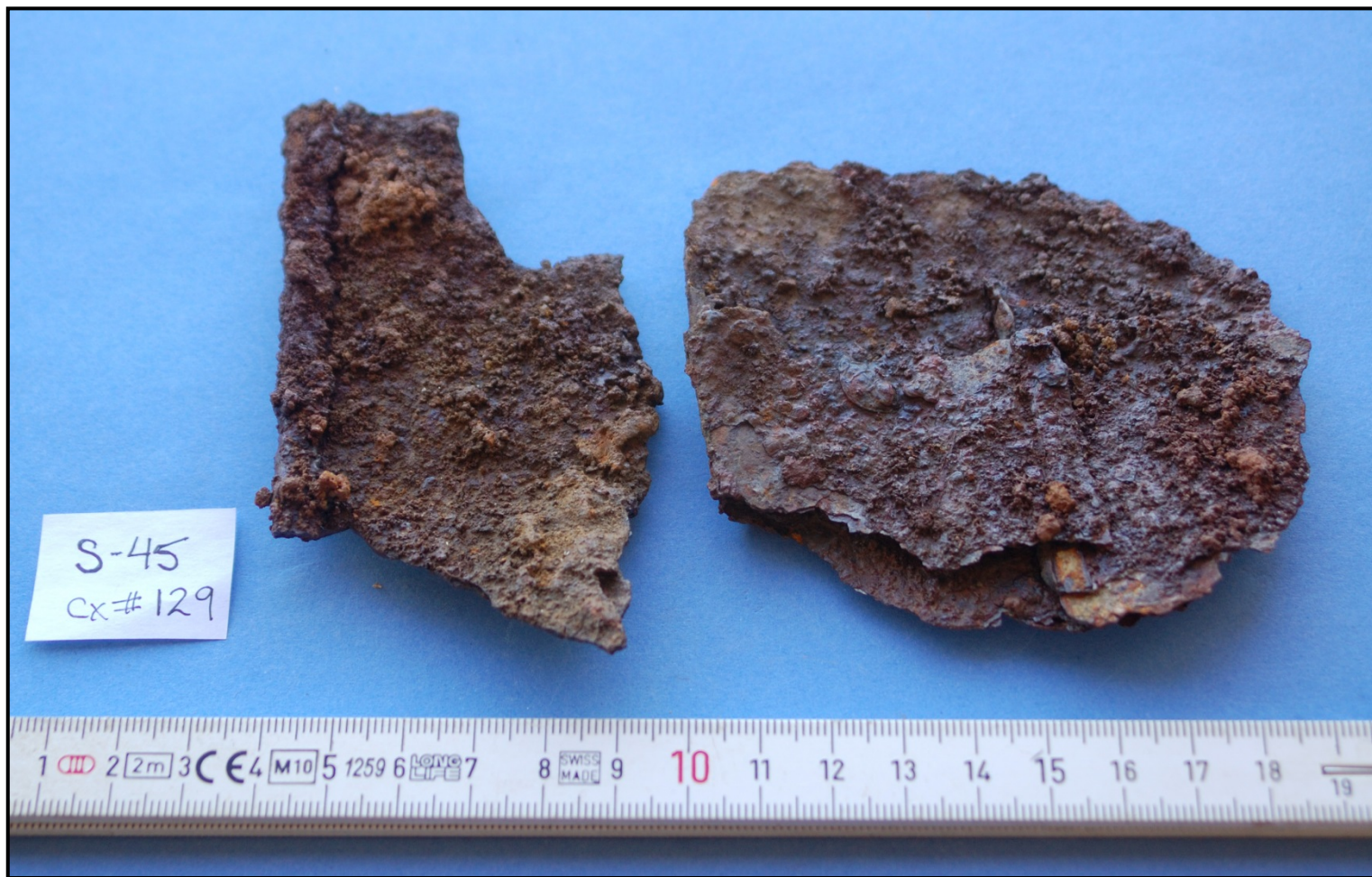
Figure 3.5: A fragment of the iron sheets interpreted as roofing material from the Wilson's house. This is an example of a piece with a folded edge.
