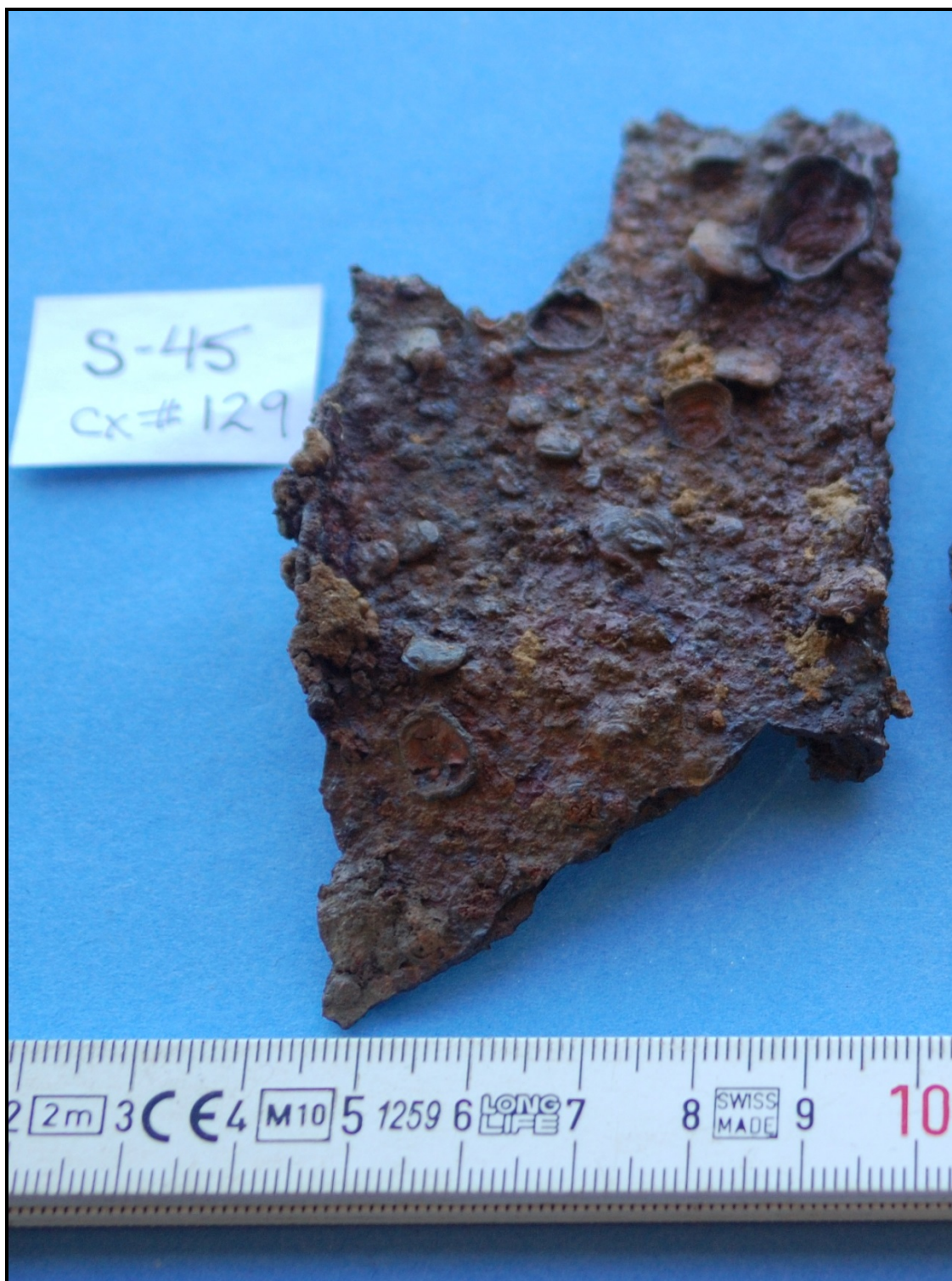
Figure 3.4: A fragment of the iron sheets interpreted as roofing material from the Wilson's house. This is an example of a piece with a rolled edge.
