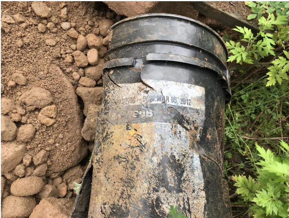
Photograph 10. Plastic Bucket Recovered from Southwest End of the Trench at a depth of 6.25 feet (1.9 m). Note date of 2012 on the bucket.
