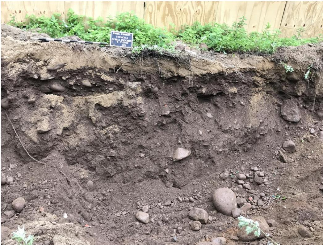
Photograph 5. South Wall Profile of the Test Trench, Showing Disturbed Fill to the Depth of 7.6 Feet (230 cmbs).
