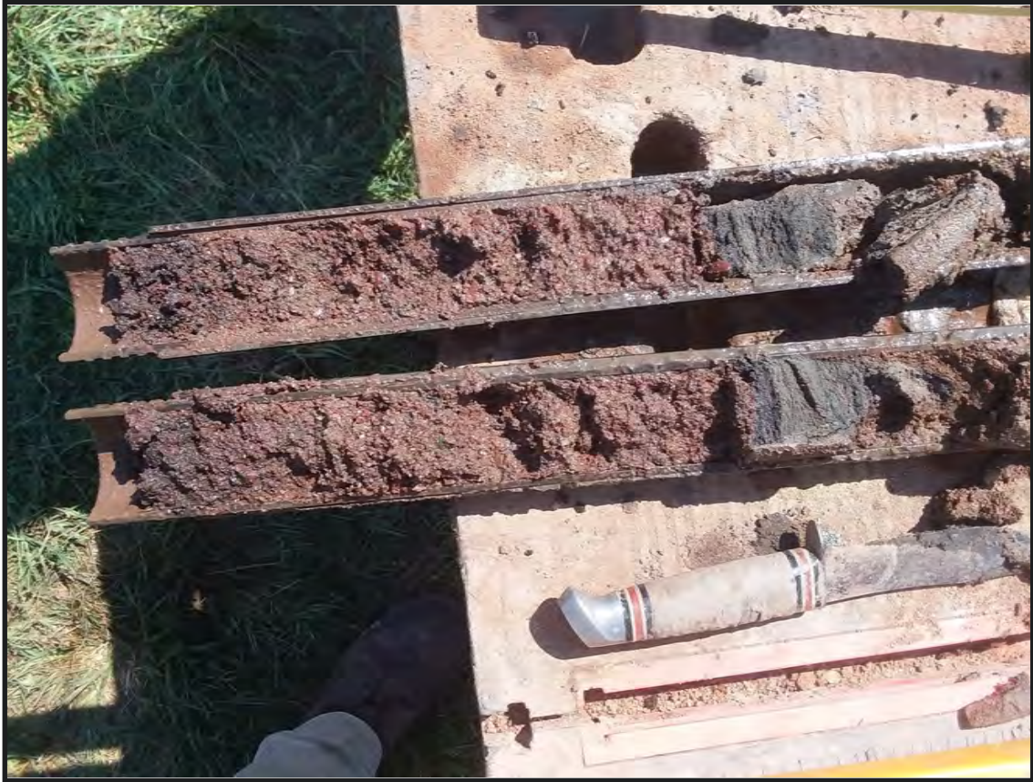
Photograph 5.9. Core sample from drill hole DH22 (New Creek Drainage), 30 to 31.5 feet below surface, slackwater alluvium sediment over alluvial bedload (Photographer: John Stiteler, September 5, 2018).
