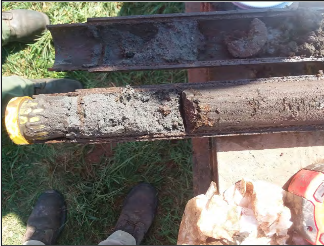
Photograph 5.5. Core sample from drill hole DH22 (New Creek Drainage), 17.5 to 19 feet below surface, lagoon deposit – silty clay with organics; sand with organics (Photographer: John Stiteler, September 5, 2018).
