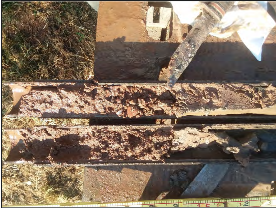
Photograph 5.11. Core sample from drill hole DH23 (New Creek Drainage), 25 to 26.5 feet below surface, alluvial silty clay over alluvial bedload (Photographer: John Stiteler, August 29, 2018).
