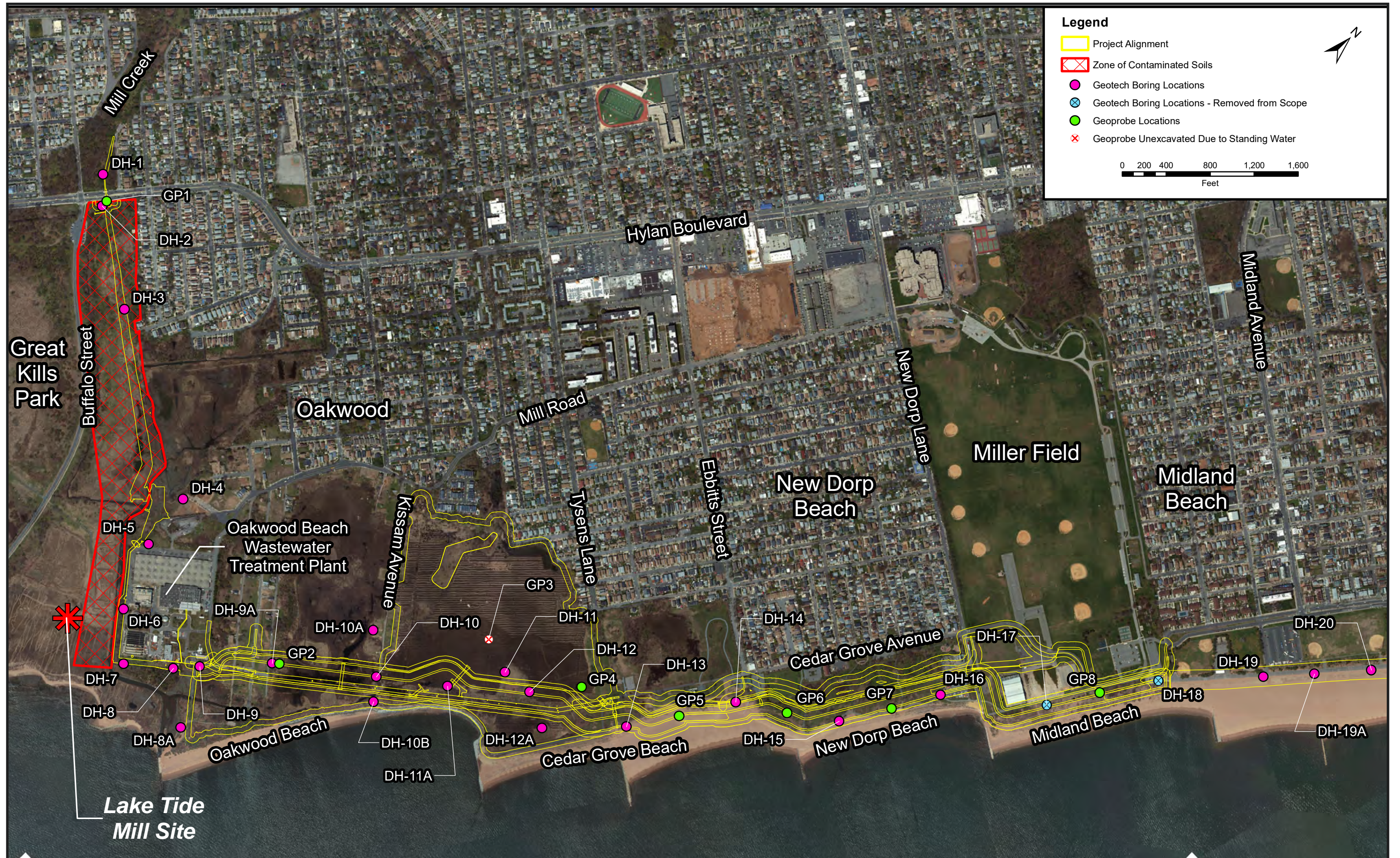
Figure 5.2a. Aerial Photograph of Project Alignment (Southwest Portion) Showing Detailed Locations of Borings. Source: New York Division of Homeland Security and Emergency 2018 and U.S. Army Corps of Engineers, New York District.
