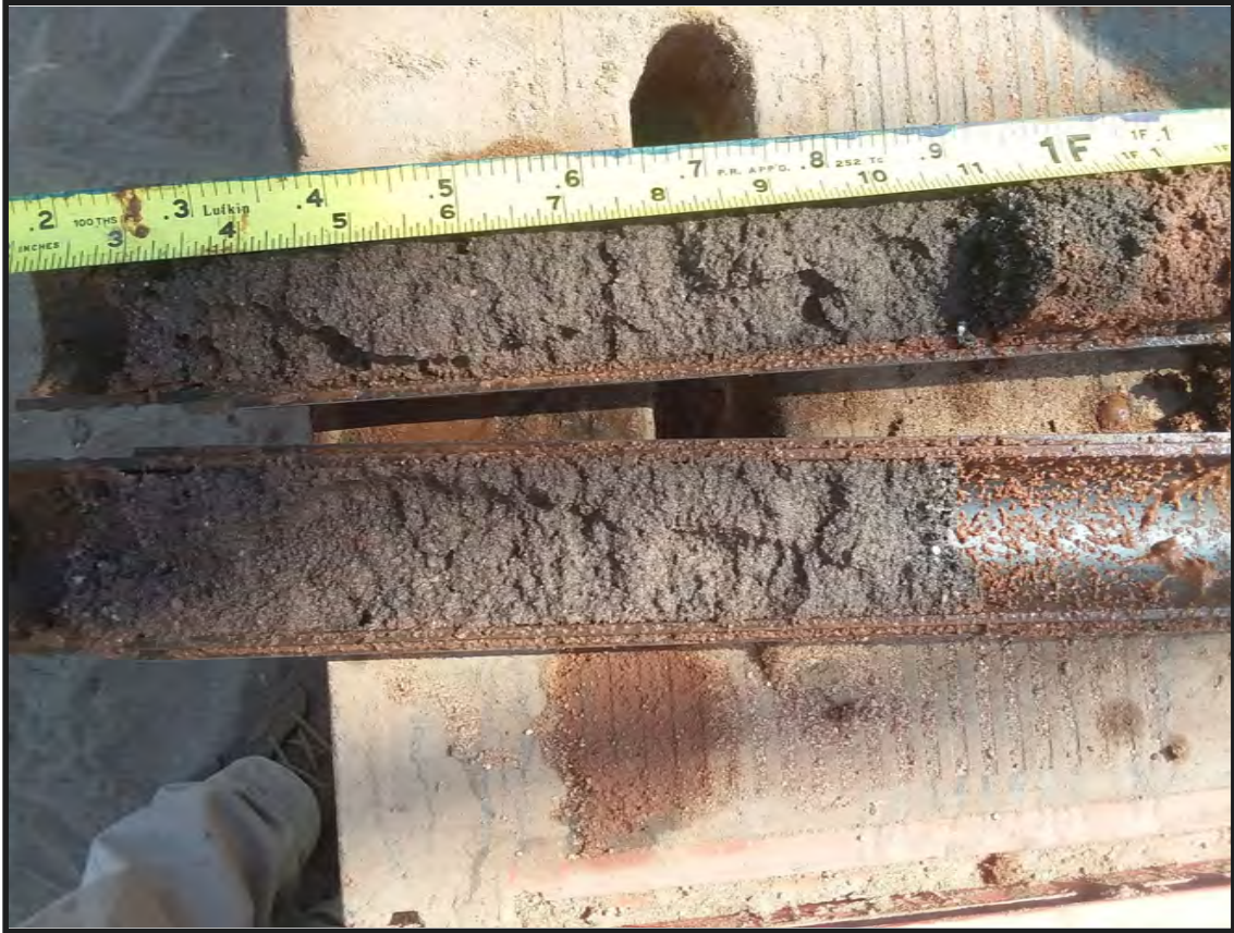
Photograph 5.4. Core sample from drill hole DH21 (New Creek Drainage), 15 to 16.5 feet below surface, backbarrier sands (Photographer: John Stiteler, September 5, 2018).
