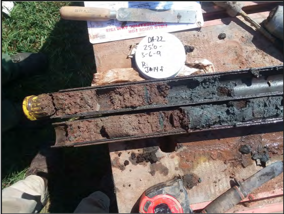
Photograph 5.7. Core sample from drill hole DH22 (New Creek Drainage), 25 to 26.5 feet below surface, basal organic-rich lagoon deposit over gravelly loam alluvium (Photographer: John Stiteler, September 5, 2018).
