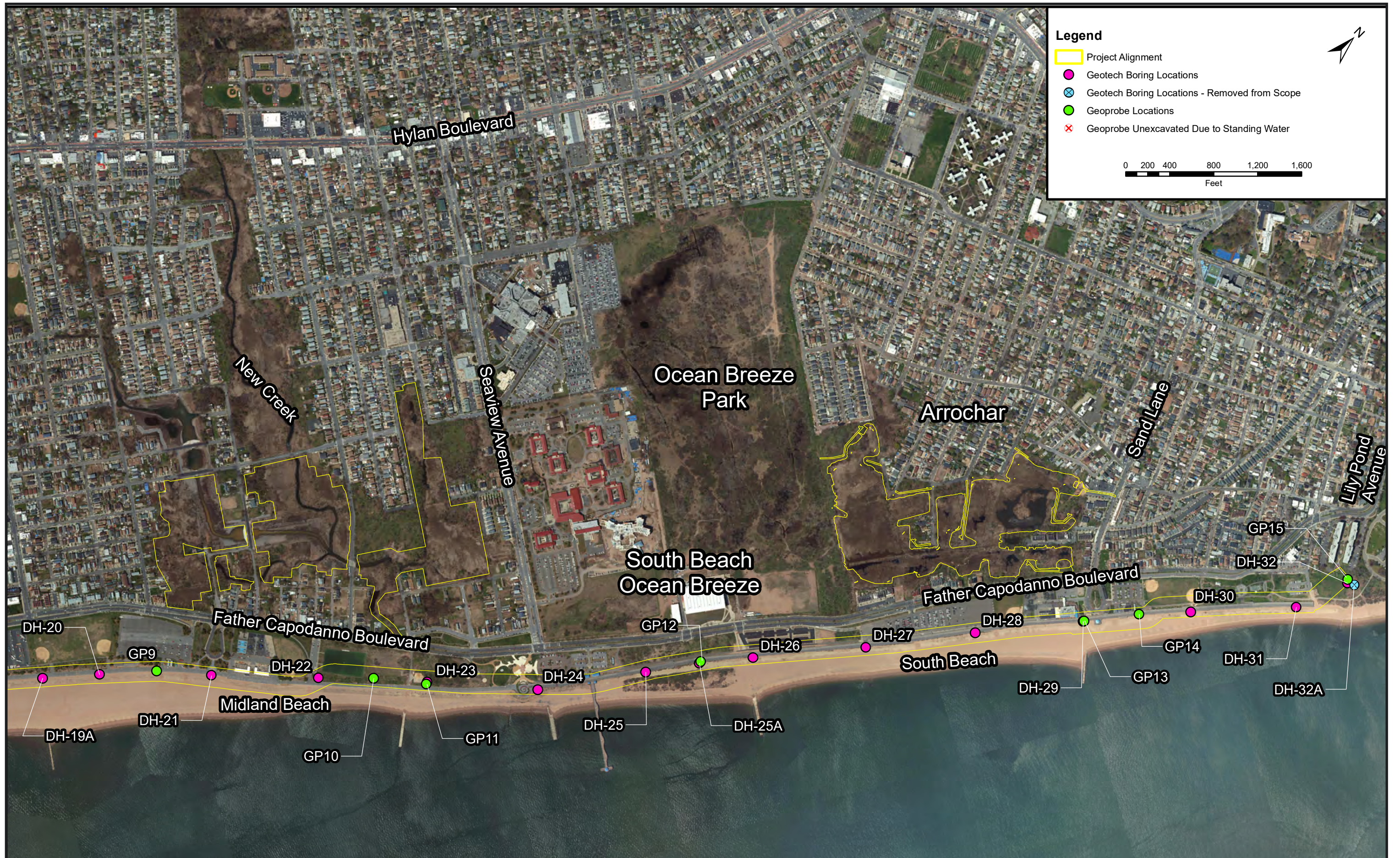
Figure 5.2b. Aerial Photograph of Project Alignment (Northeast Portion) Showing Detailed Locations of Borings. Source: New York Division of Homeland Security and Emergency 2018 and U.S. Army Corps of Engineers, New York District.
