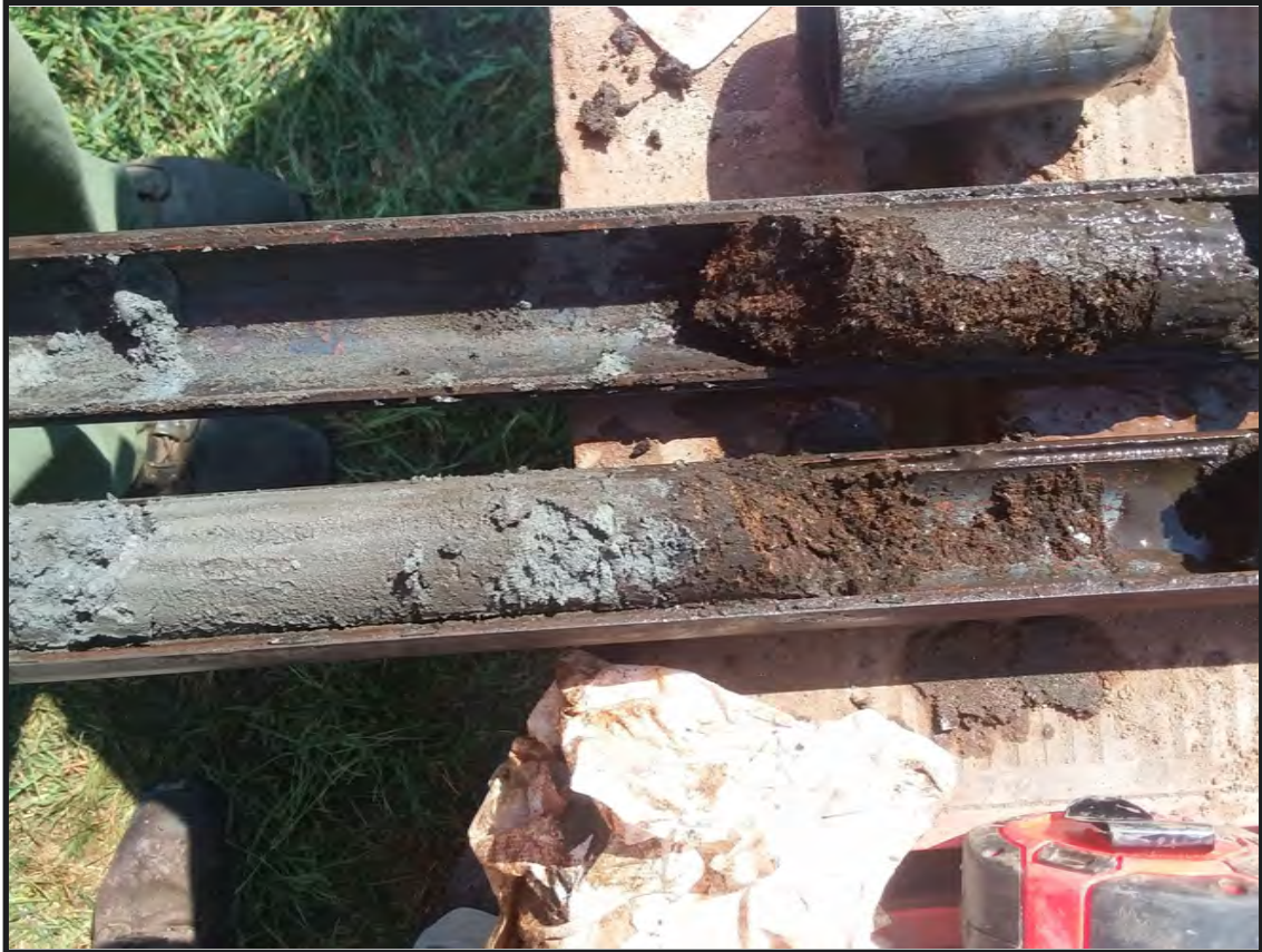
Photograph 5.6. Core sample from drill hole DH22 (New Creek Drainage), 22.5 to 24 feet below surface, basal lagoon peat over gleyed sandy clay (Photographer: John Stiteler, September 5, 2018).
