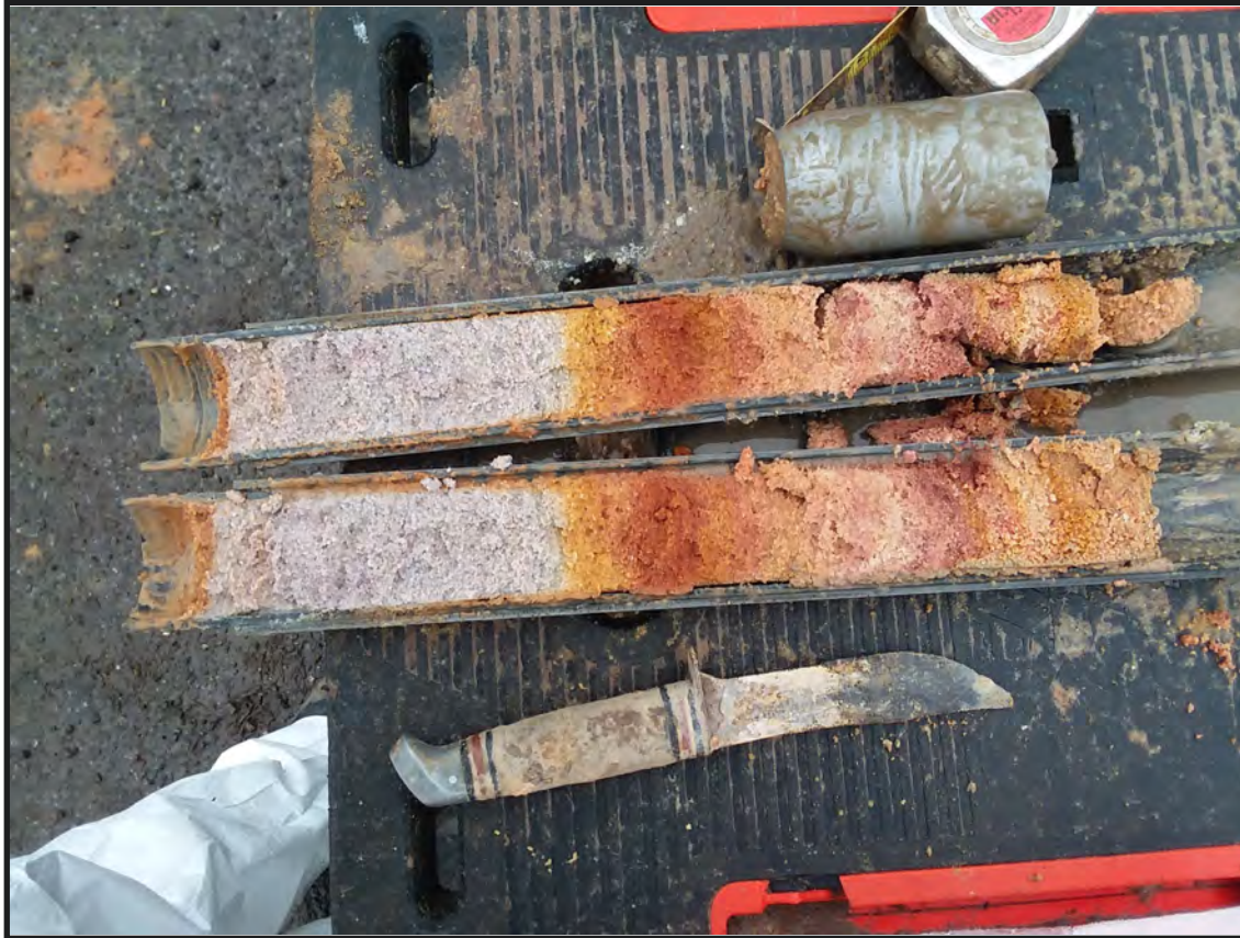
Photograph 5.3. Core sample from drill hole DH10 (Oakwood Beach Marsh), 115 to 116.5 feet below surface, Cretaceous sand and clay of the Raritan Formation (Photographer: John Stiteler, November 3, 2018).
