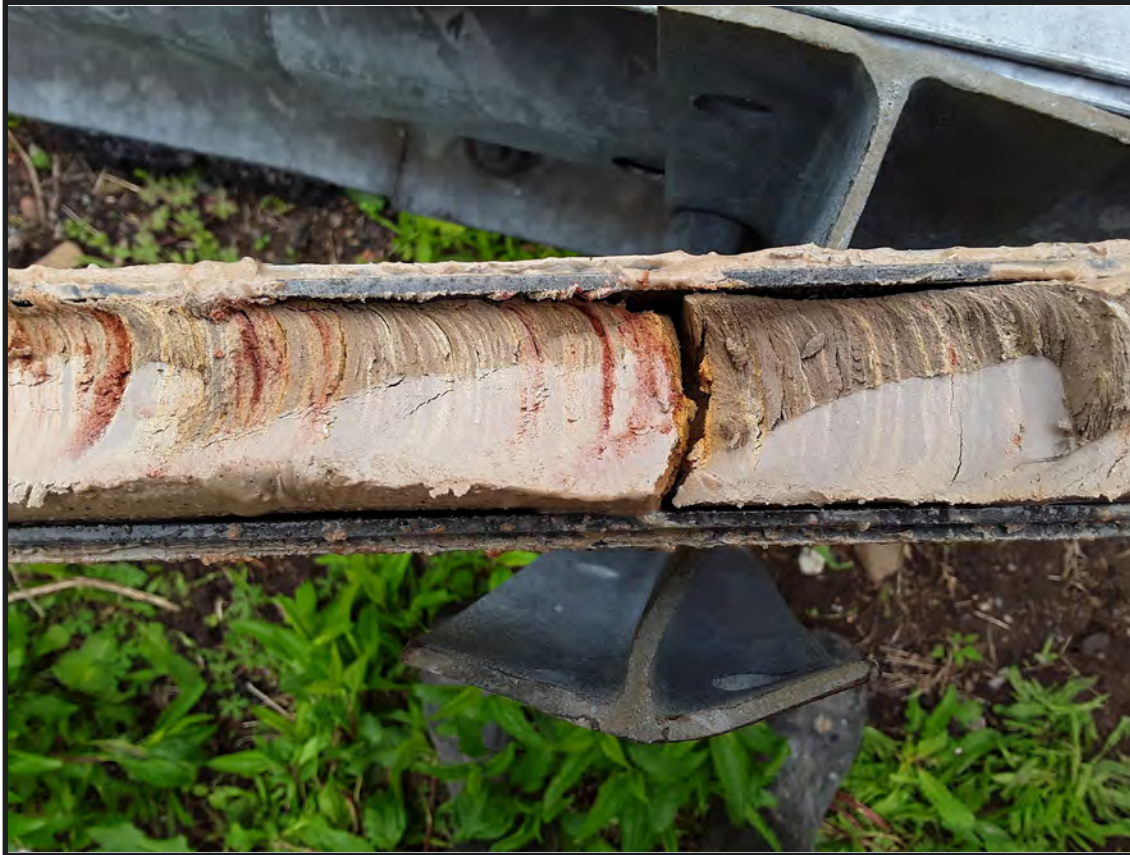
Photograph 5.1. Core sample from drill hole DH6 (Oakwood Beach Marsh), 117.5 to 119 feet below surface, Cretaceous sand and clay of the Raritan Formation (Photographer: John Stiteler, April 30, 2019).
