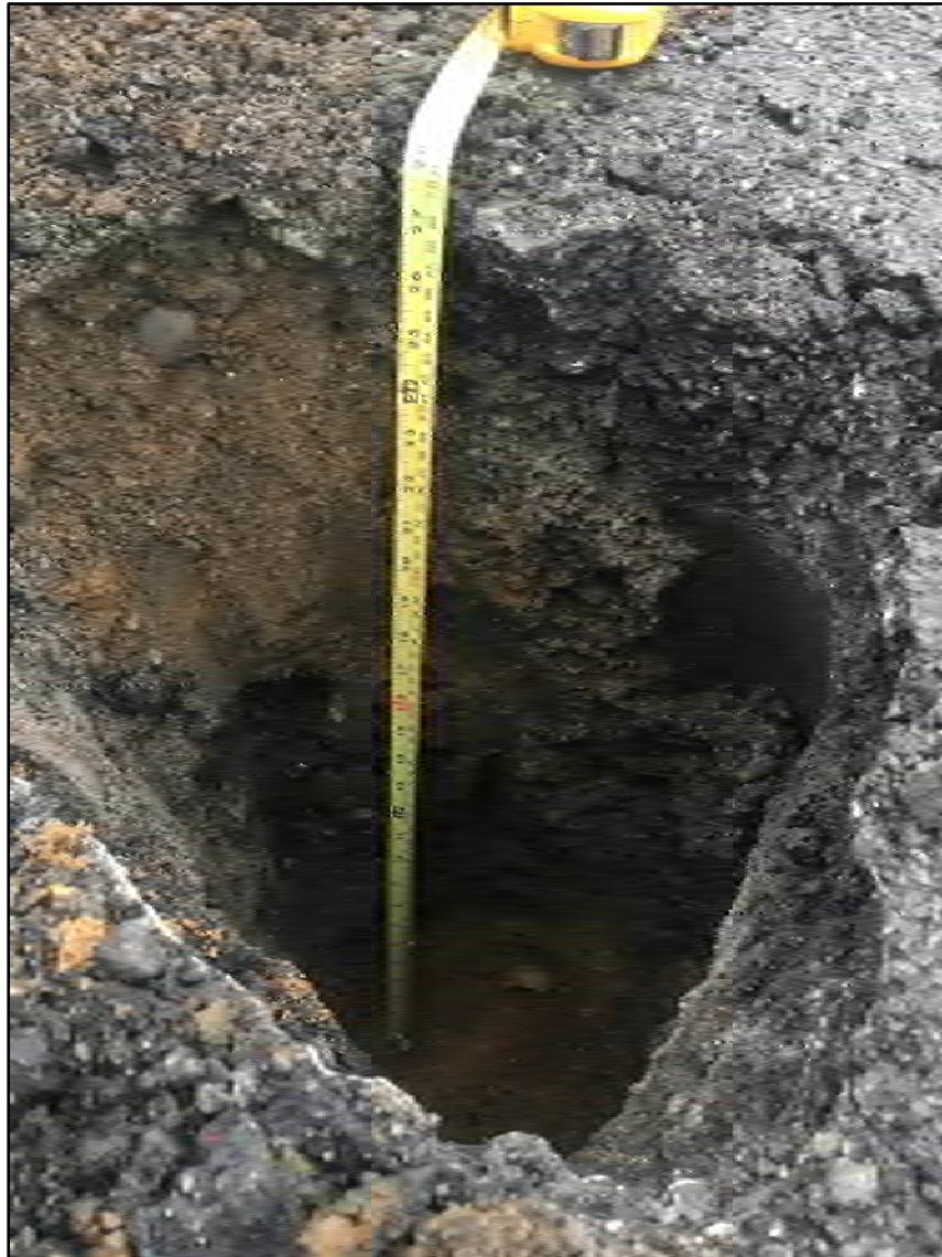
Photograph 4.5 Posthole from northern half of construction fence line, excavated approximately 2 feet below grade, fill soils encountered.
