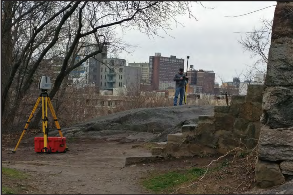
Photograph 3.4. View facing north showing GPS surveying of the datum for the topographic scan (Photographer: James Lee, March 2017 [HRI Neg.#17013/D1:024]).
