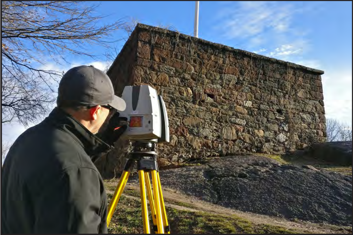
Photograph 3.1. View facing northeast showing digital laser scanning equipment being set up southwest of the blockhouse to scan the western and southern facades (Photographer: James Lee, March 2017 [HRI Neg.#17013/D1:002]).
