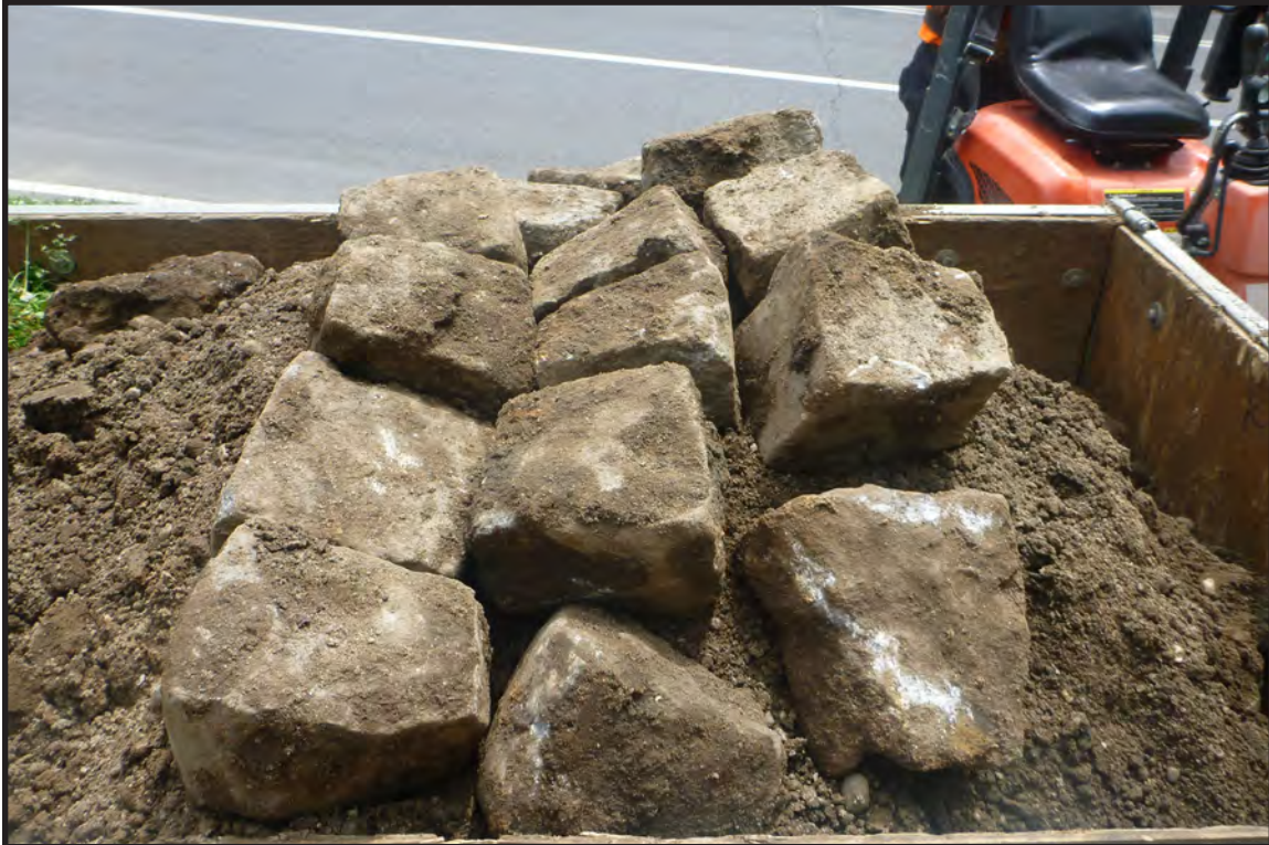
Photograph B.9. View facing east showing an example of stone setts that were excavated from SLB #10 (Photographer: Joshua Butchko, May 2021 [HRI Neg.#21036/D2:042]).
