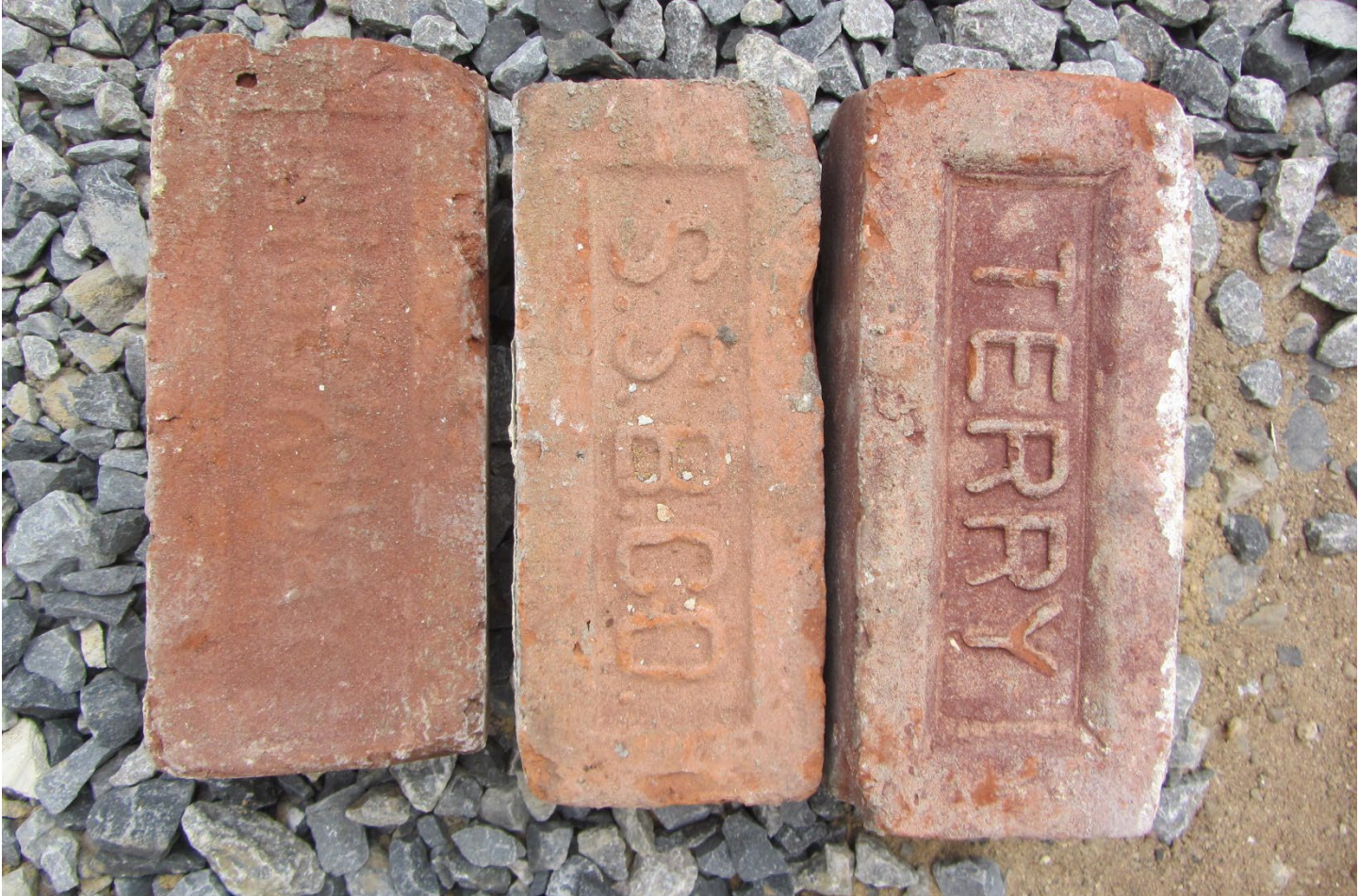
Photograph 7: Representative bricks removed from interior walls of Vault B.
