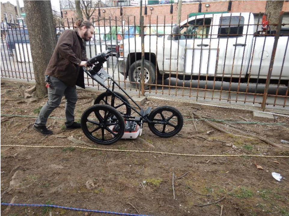
Photo 8. GPR survey of the west lot of the New Lots Library.
