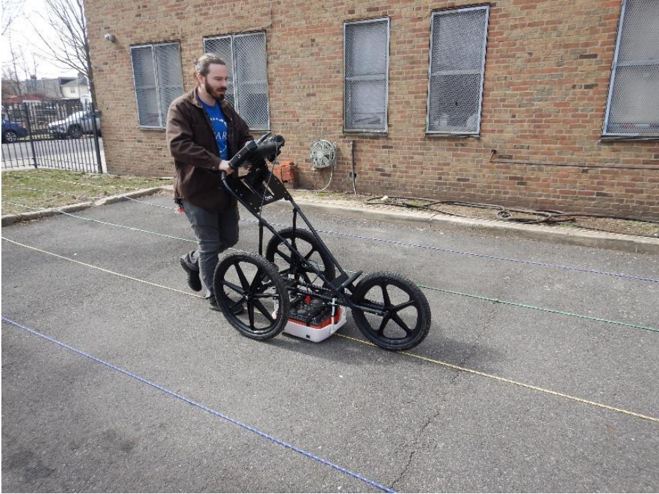
Photo 7. GPR survey of the east parking lot.
