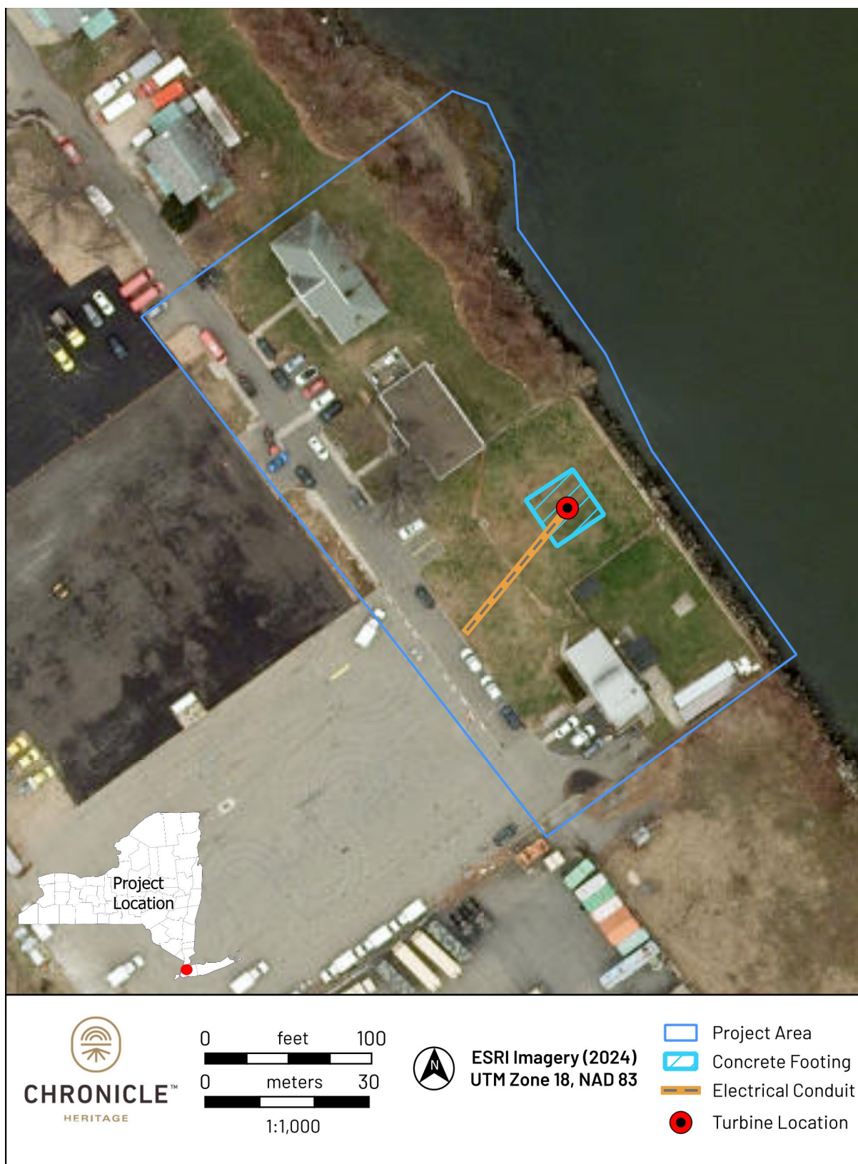
Figure 1-2. Detail map of Project area, showing proposed location of wind turbine, footing, and electrical conduit (Esri 2024).
