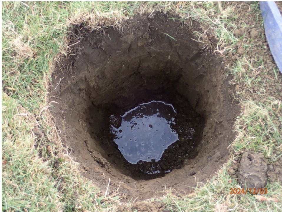
Photograph 4. Water table at the bottom of ST 3. (LC 12/3/2024)
