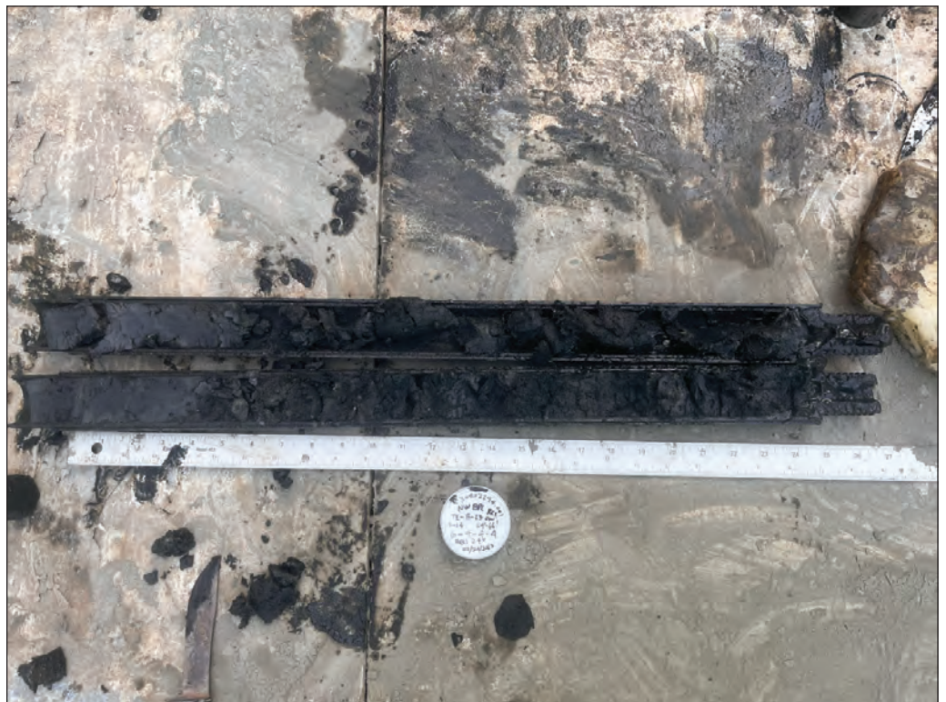
Photograph 2: Boring B-23, 64 to 66 feet bgs (-52 to -54 feet): typical estuarine organic silty clay, contained wood, much coal cinder
