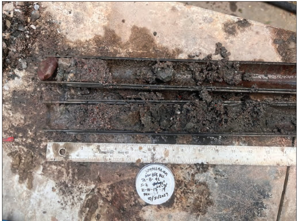
Photograph 6: Boring B-42, 29-31 feet bgs (-21 to -23 feet) gravelly glacial outwash sand, reworked by wave action, upper zone stained by overlying organic-rich estuarine sediments
