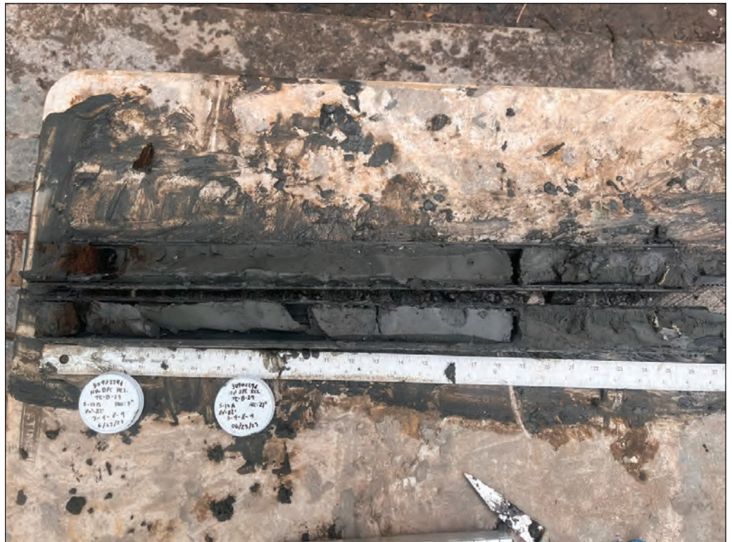
Photograph 4: Boring B-29, 80-82 feet bgs (-64 to -66 feet) typical estuarine organic silty clay, contained shell; peat visible near top of sample, no historic period markers noted
