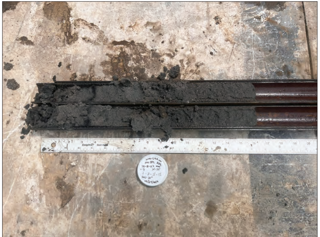
Photograph 1: Boring B-23, 30 to 32 feet below ground surface (bgs) (-18 to -20 feet): typical sand fill, including coal cinder and fine shell
