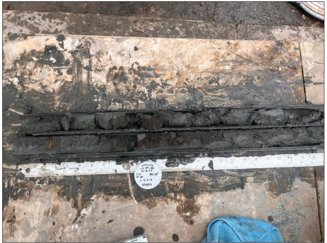
Photograph 5: Boring B-29, 82-84 feet bgs (-66 to -68 feet) typical estuarine organic silty clay, contained shell; peat visible near middle of sample, no historic period markers noted
