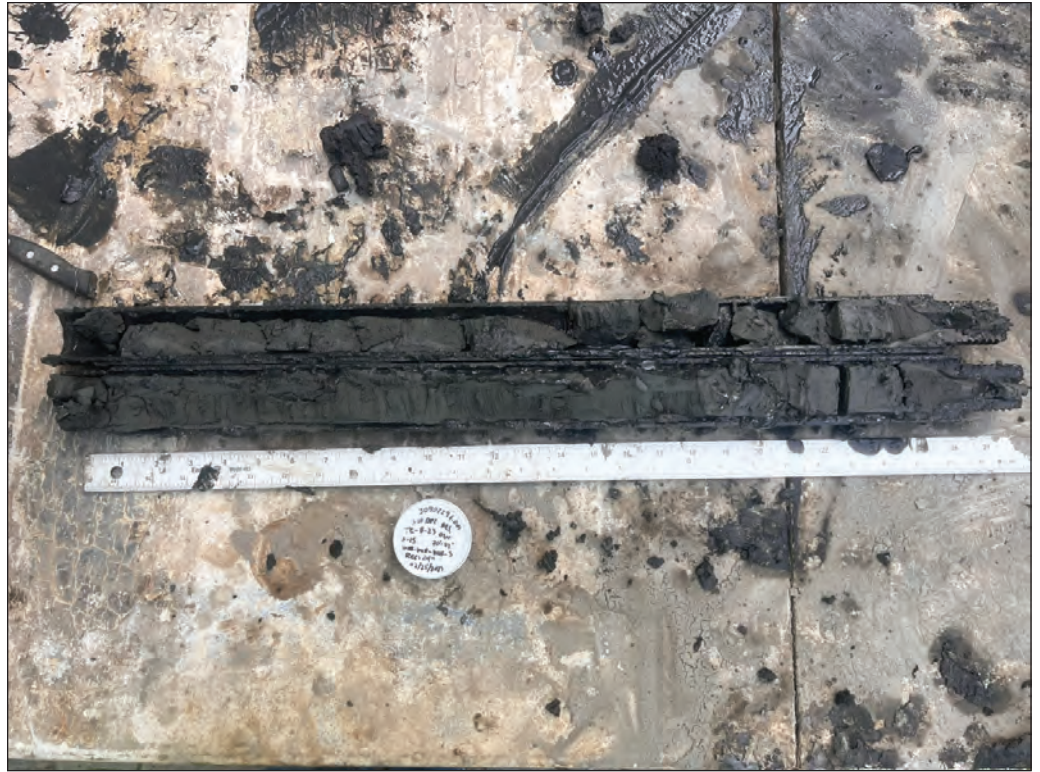
Photograph 3: Boring B-23, 70 to 72 feet bgs (-58 to -60 feet): typical estuarine organic silty clay, contained wood, no Historic markers noted
