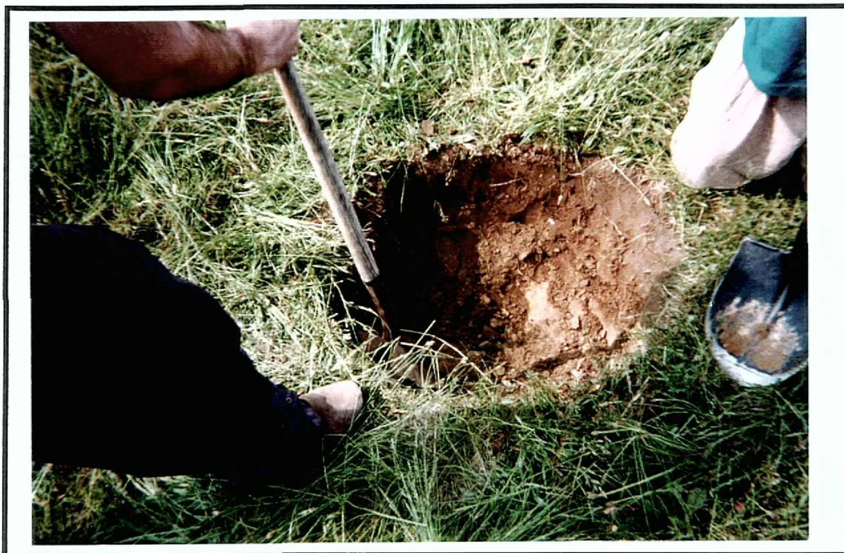
Photo 7: Interface between topsoil and fill stratum.
