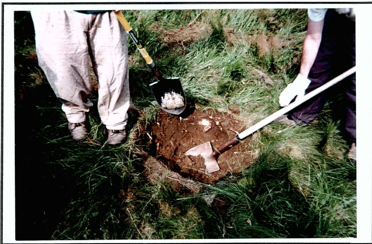
Photo 9: The site exhibited 8' to 10' of topsoil layer deposited over fill to create convent garden.
