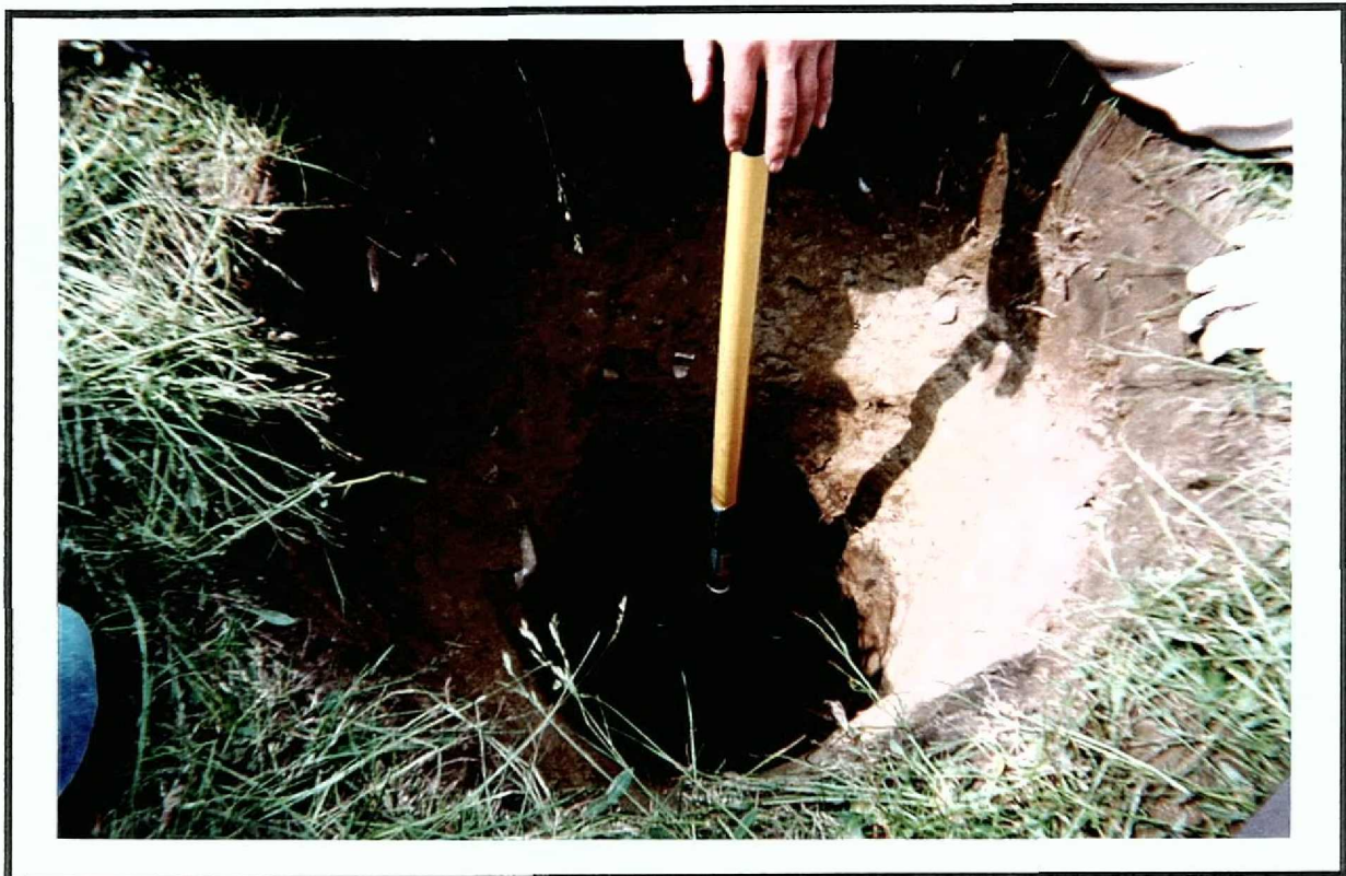
Photo 5: Stratigraphic control test showing topsoil, fill layer, and historic plowzone.
