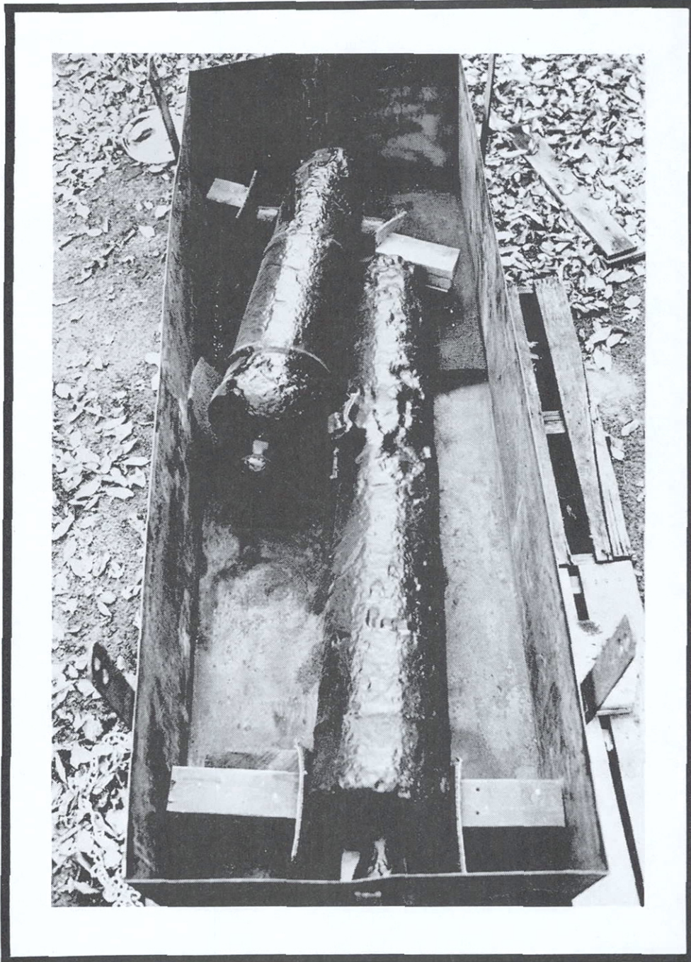
PLATE 3. Two Cannon (C and E) Broken Through the Chase
