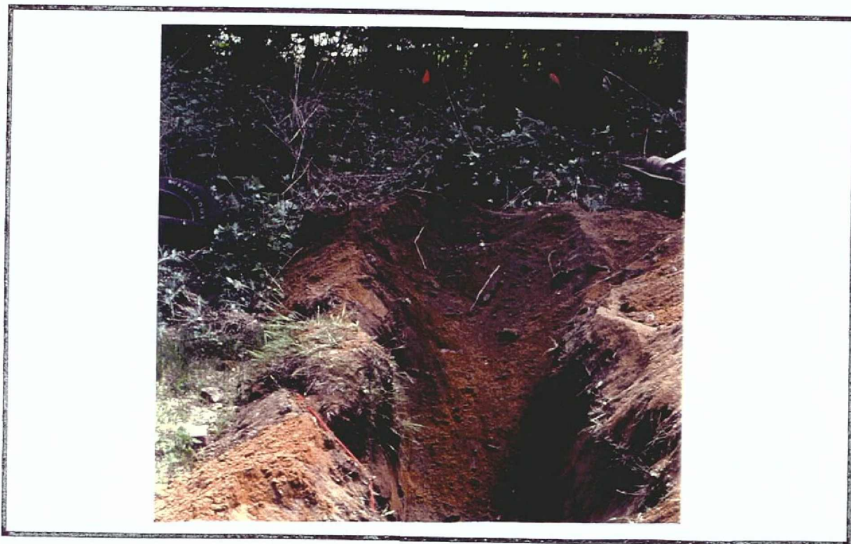
Photo 20: Extremely soft sand filled Lot 23 to a depth of six feet. The dark yellow sand failed to maintain the walls of the test trench.
