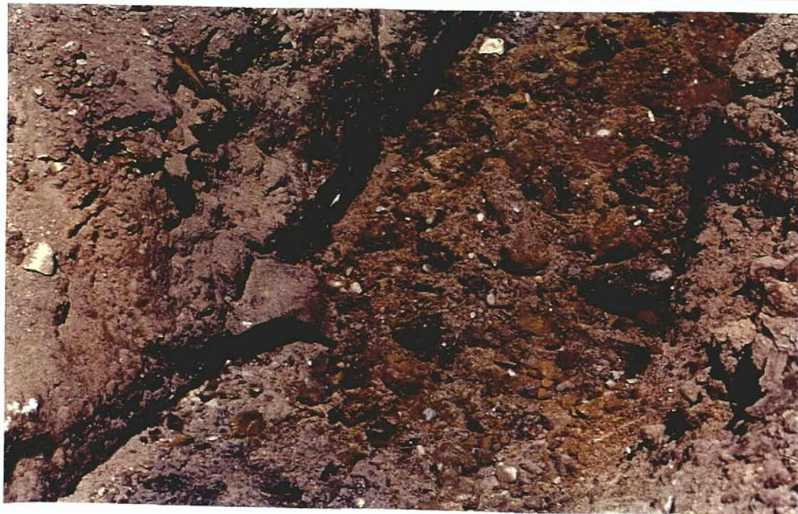
Photo 3: Urban soils mixed with destruction debris persisted to the bottom of trenches on Lots 11 and 13 to a depth of up to 10'.
