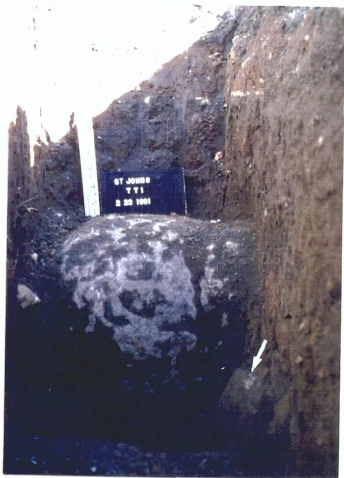
3 Boulder exposed at north end of TT1 approximately 34 in. below the parking lot surface. A smaller rock can be seen in the east wall to the right (arrow).
