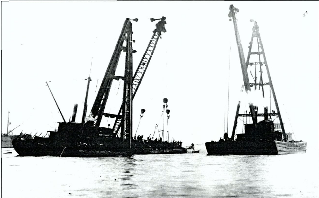
Figure 8. Undated photograph of two A-frame crane barges involved in what appears to be a salvage operation. Note scow hulls, the machinery cabin, as well as the numerous crane stays on the barge to the left. These stays and their corresponding chain plates where they attach to the hull are a distinguishing characteristic of this vessel type (courtesy of the South Street Seaport Museum).
