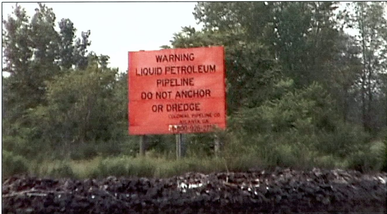
Figure 78. Photograph of pipeline sign indicating source of Anomaly 110.
