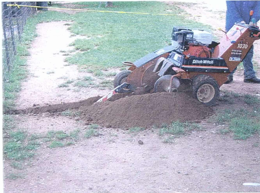
Figure 08: Trench cutting machine for utility lines
