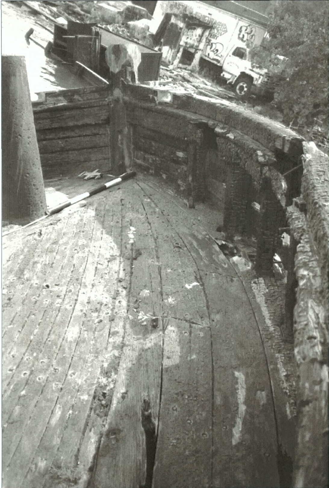
Figure 7-73. Main deck forward, showing yacht style deck plank. Note larger timbers of changing dimension adjacent to waterway.
