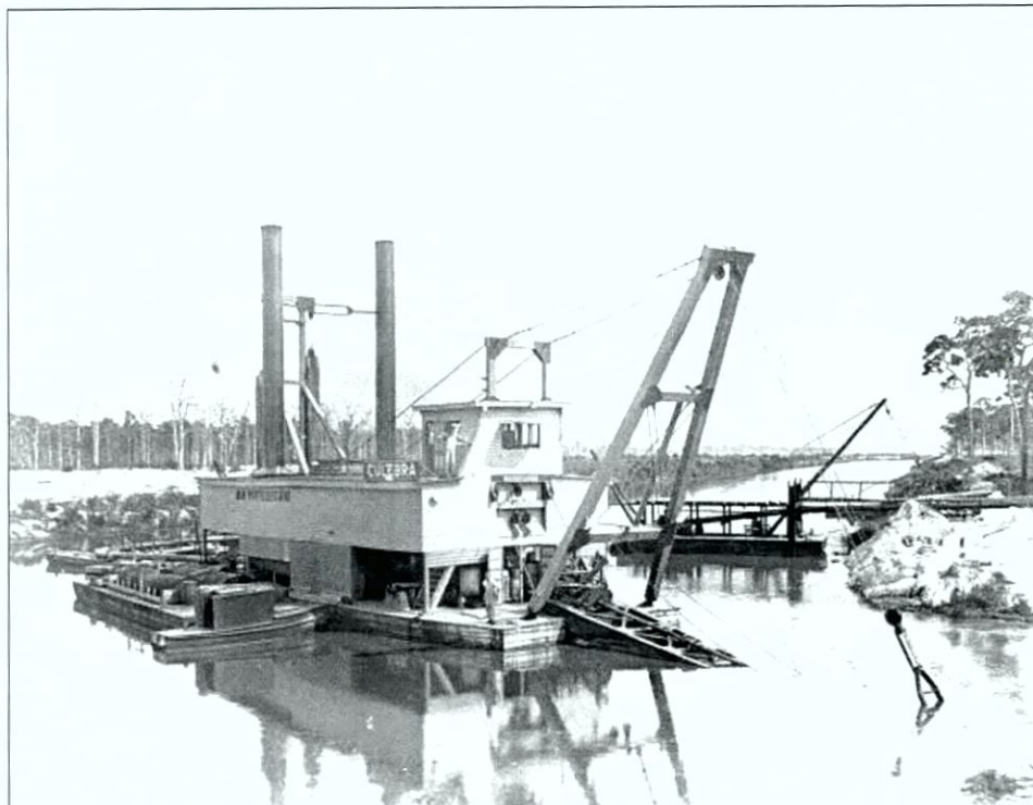
Figure 4-09. Dredge Culebra with boom lowered into working position (photo courtesy of the Florida Photographic Collection).
