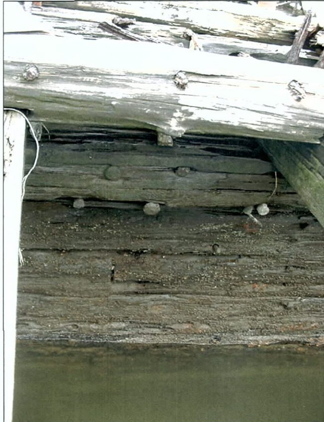
Figure 6-82. Starboard side looking starboard (east) showing extant mold ceiling. Note composite shelf just below deck beams.
