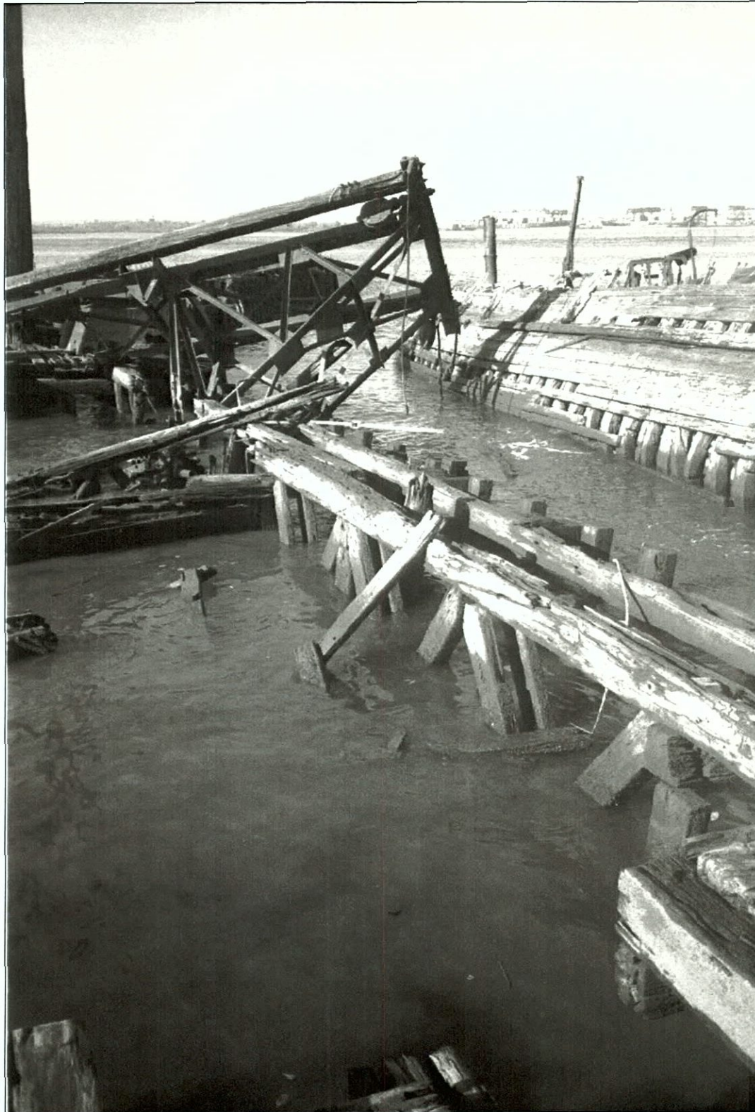
Figure 4-31. Port side framing. Note aft bulkhead, center left. View to the north (aft).
