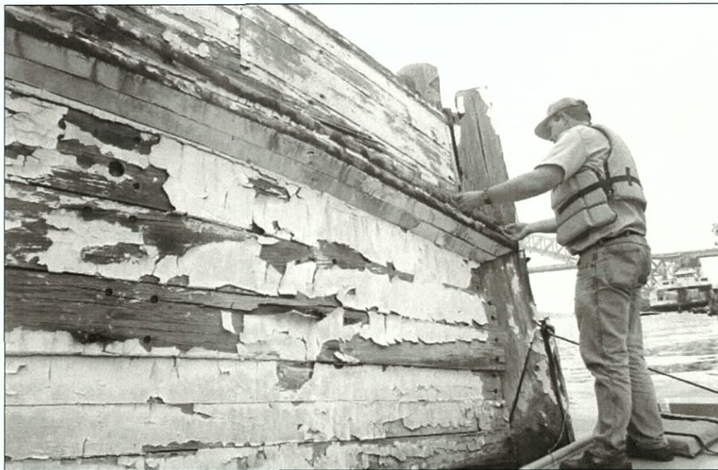
Figure 7-55. Starboard side of bow, showing main rub rail construction. View to the southeast.
