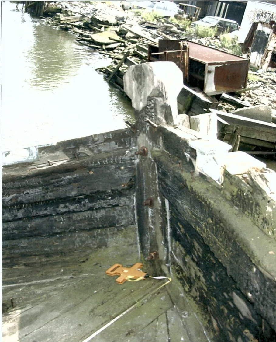
Figure 7-45. Fish Hawk stem assembly from foredeck, looking forward and south.
