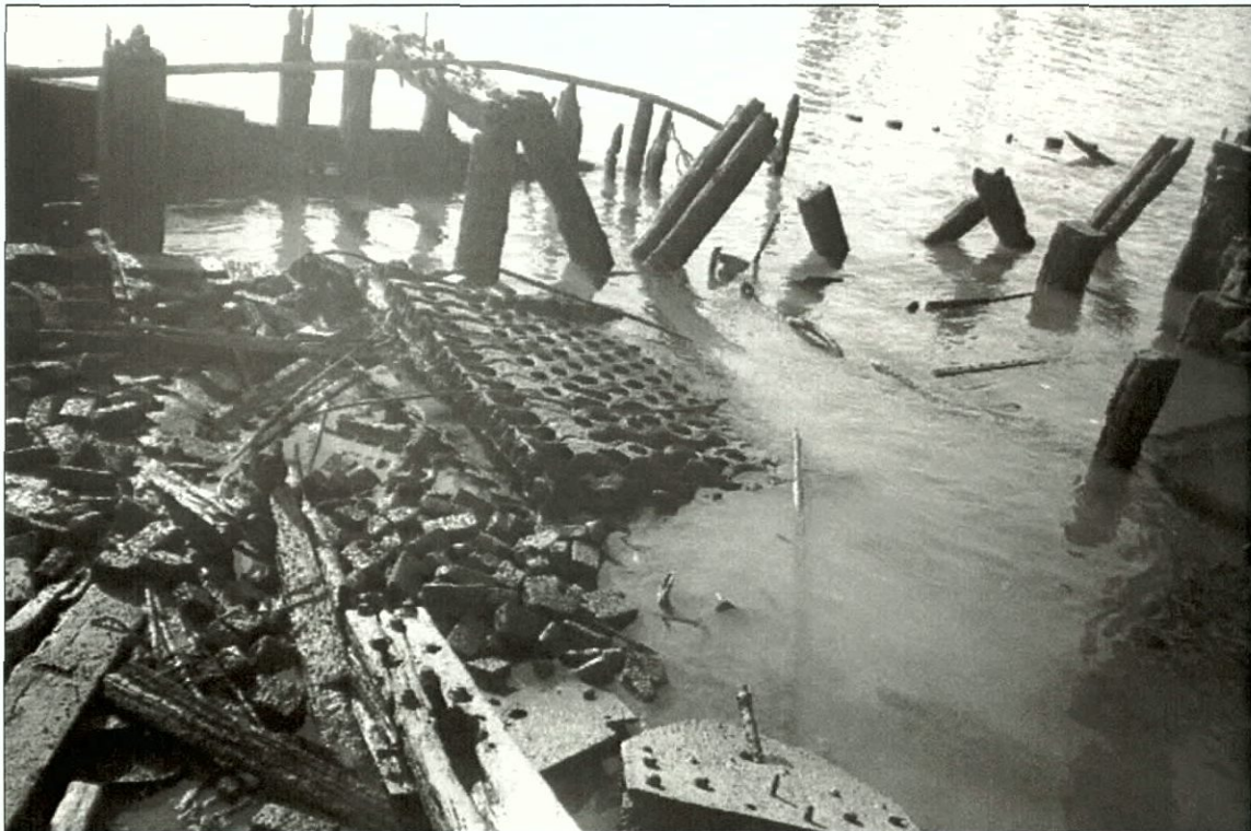
Figure 4-33. Starboard side, view to the southwest. Note diagonal truss timbers, vertical stanchions, and athwartships beams tying the trusses in to the side of the vessel.
