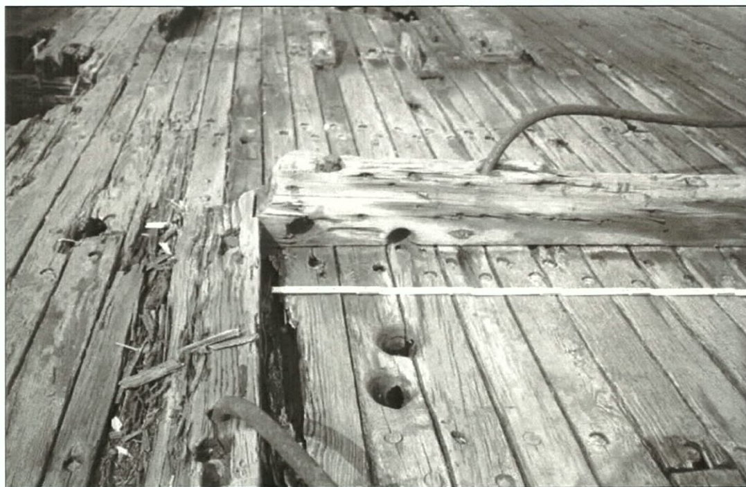
Figure 7-85. Aft pilothouse bulkhead remains showing steering cable passages. View to the north (aft).
