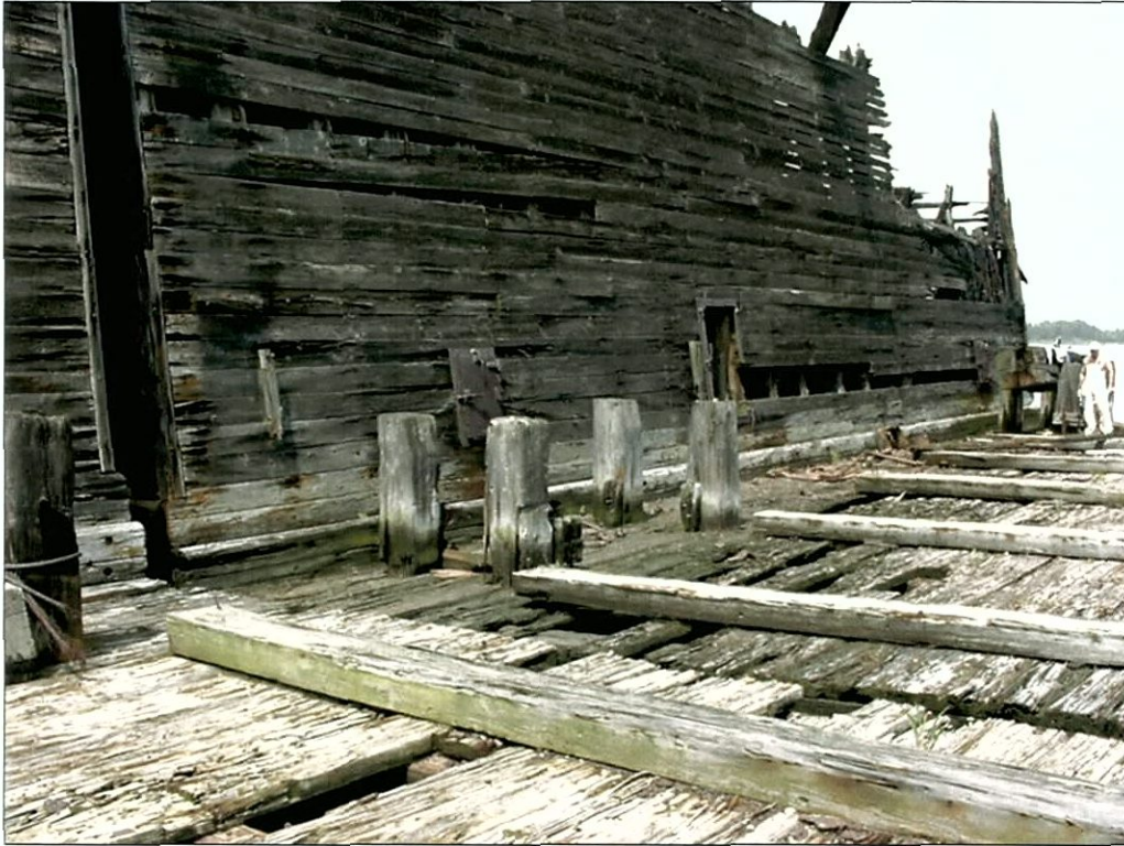
Figure 5-80. View from aft looking toward port bow, showing placement of bilge block stringers and port aft bitt.
