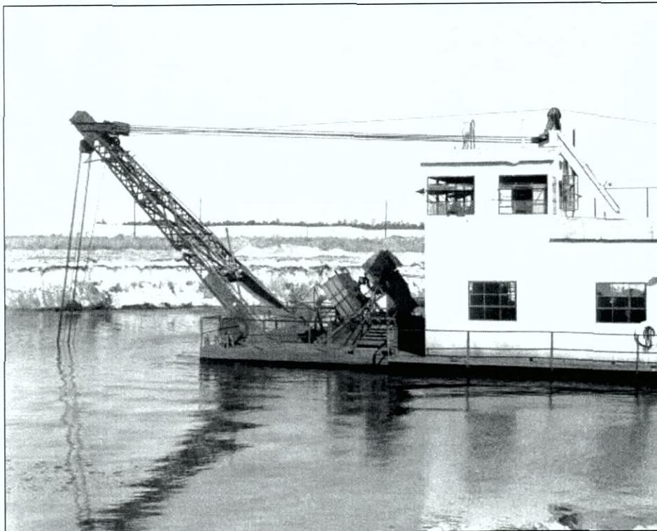
Figure 4-17. Detail of bow of cutterhead dredge Starke , Florida, circa 1957. Note well and cable arrangement for raising and lowering the boom (photo courtesy of the Florida Photographic Collection).
