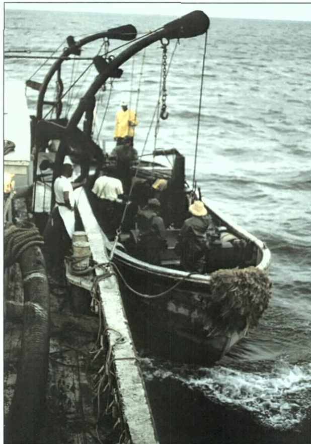
Figure 7-17. Modern seine boat being lowered from the stern of a menhaden trawler (courtesy of NOAA).
