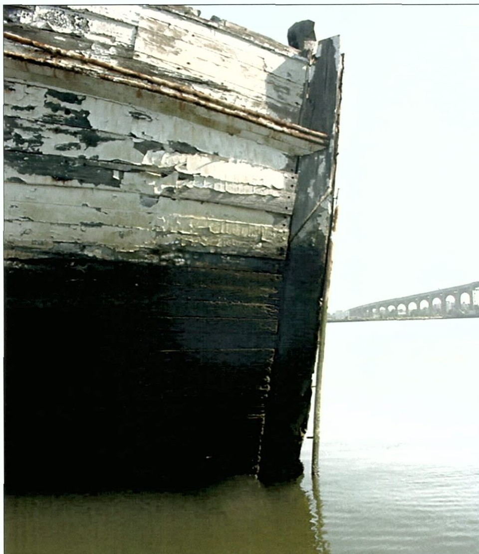
Figure 7-42. Fish Hawk stem assembly from starboard side, looking east. Note plain scarph on stem timber, just below rub rail.
