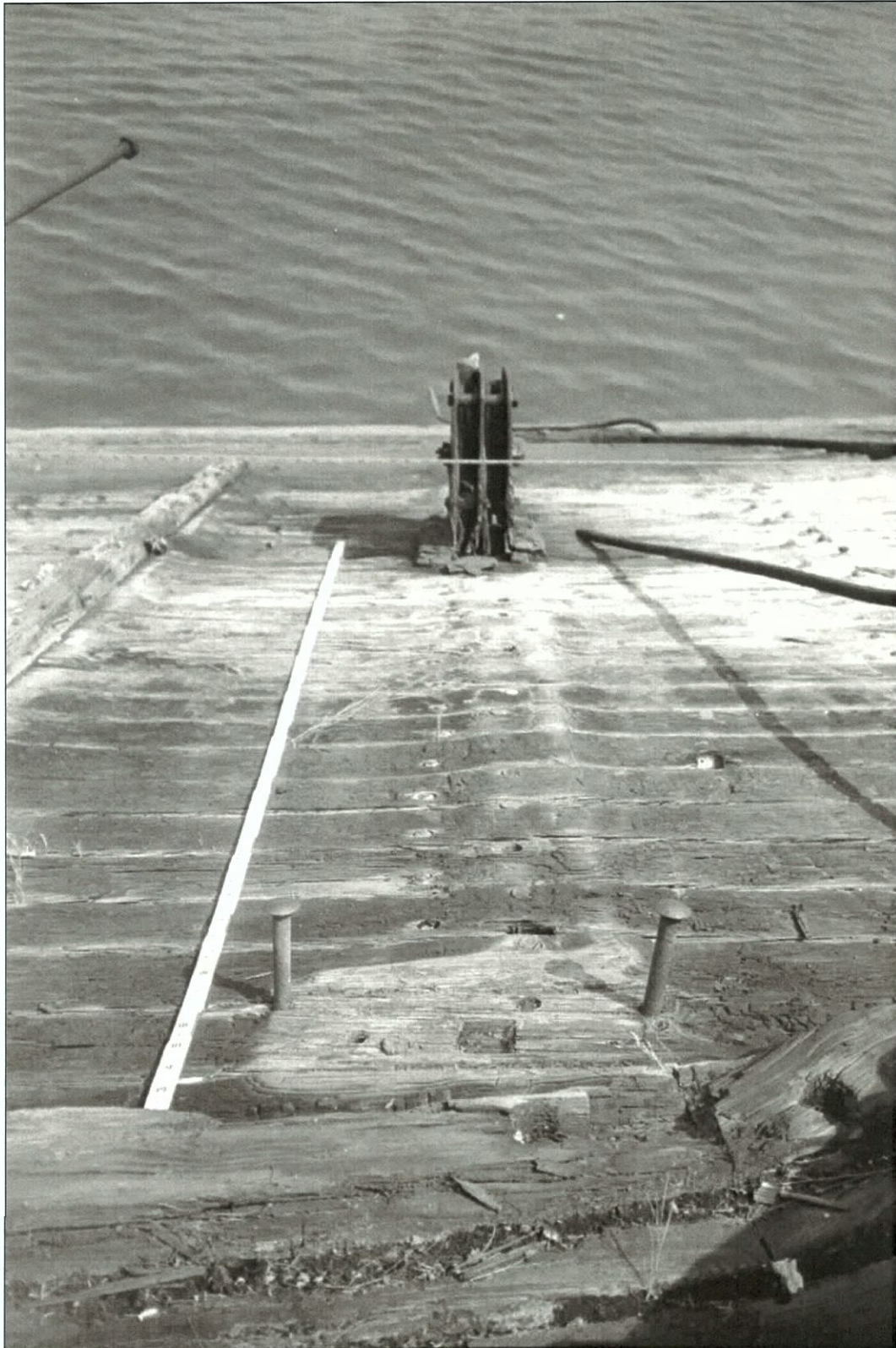
Figure 7-83. Forward section of pilothouse showing remains of steering gear. View to the east (starboard). Note mounting pad for pulley in foreground.
