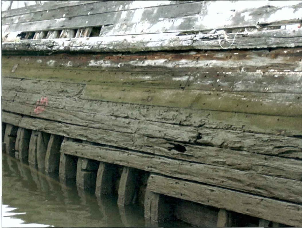
Figure 7-49. Starboard side view, looking northeast, of midship section showing exposed framing at the turn of the bilge.
