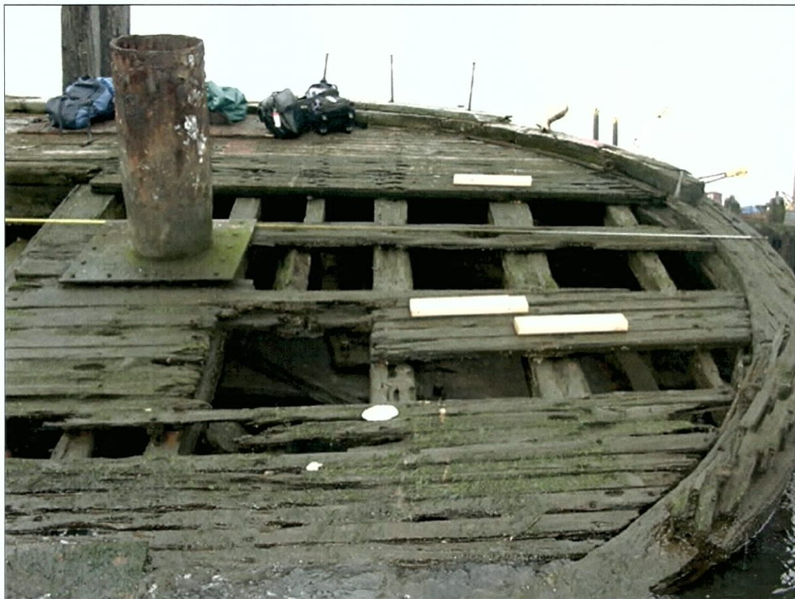
Figure 7-74. View looking starboard (west) showing quarterdeck planking.
