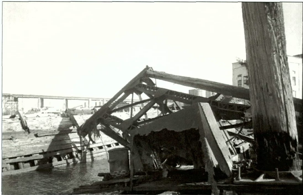
Figure 4-61. Spud box and a pole, and collapsed A-frame at the aft end of the vessel. View to the southeast (forward).
