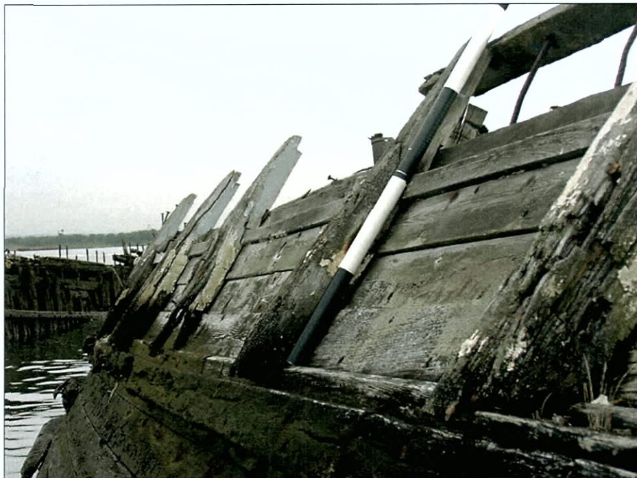
Figure 7-81. Port side of vessel showing quarterdeck rail stanchions. View to the north (aft).
