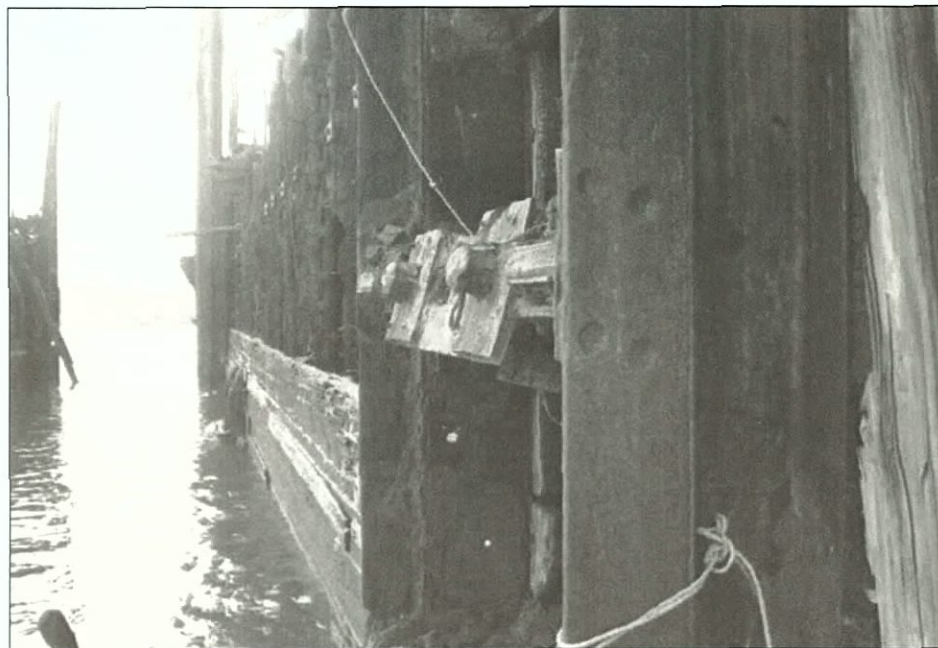
Figure 5-167. Close-up of starboard forward spud. Note truck. View to the south (aft).
