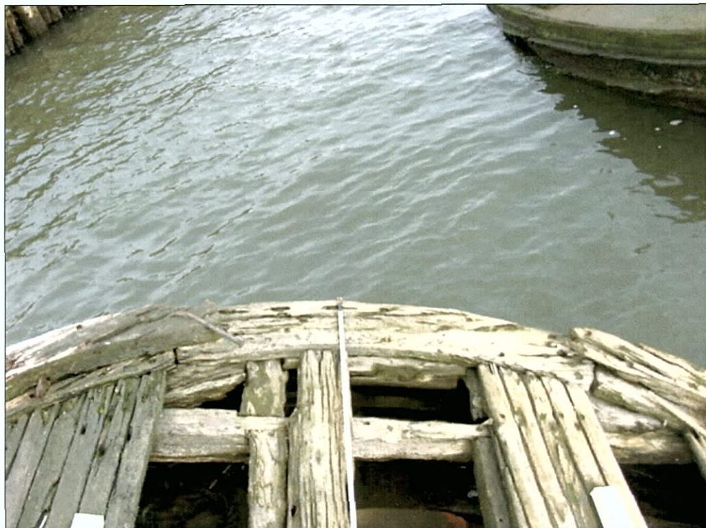
Figure 7-48. Stern detail showing timbers used to construct stern. Photo taken looking aft (north).
