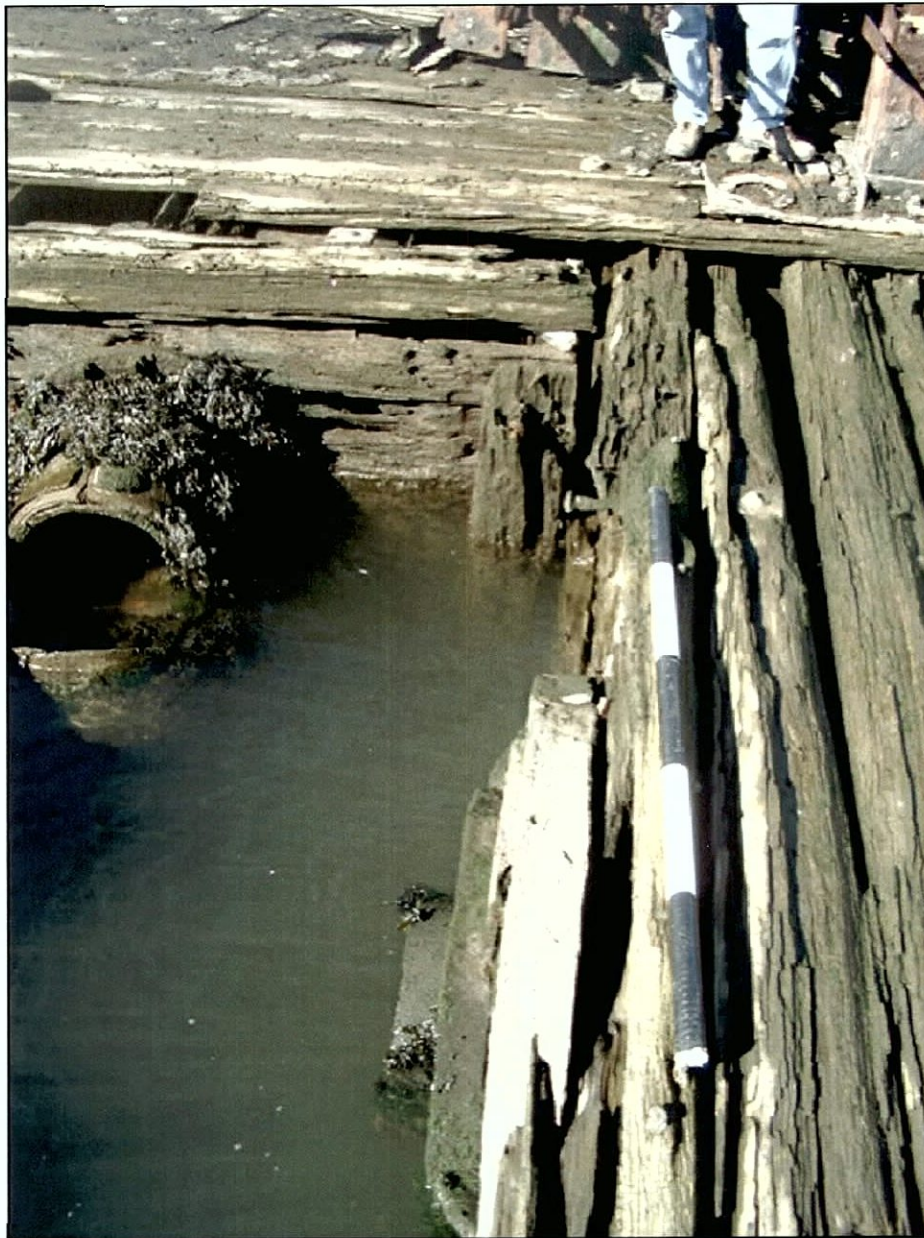
Figure 4-37. Starboard hull extension framing and planking. Note also suction pipe along centerline of vessel. View to the north (aft).
