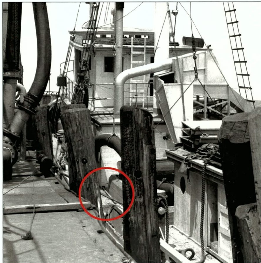
Figure 7-84. Mermentau port side. Note small pipe on deck just outboard of main cargo hatch, containing steering cable (photo courtesy of Bob Cubbage).
