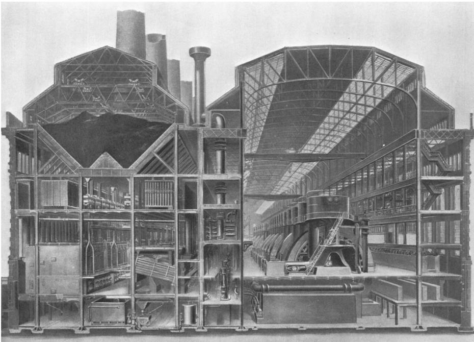
**IRT Powerhouse, section drawing showing boiler house (left) and operating room (right), c. 1904**
