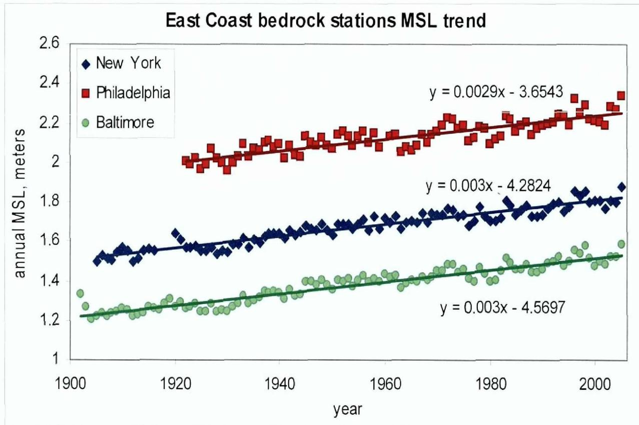
Figure 3.3. Comparison of tide gauges of long-term bedrock-founded sites. Each site shows a rate of rise of 2.9 to 3.0 mm/yr (0.12 in/yr).
