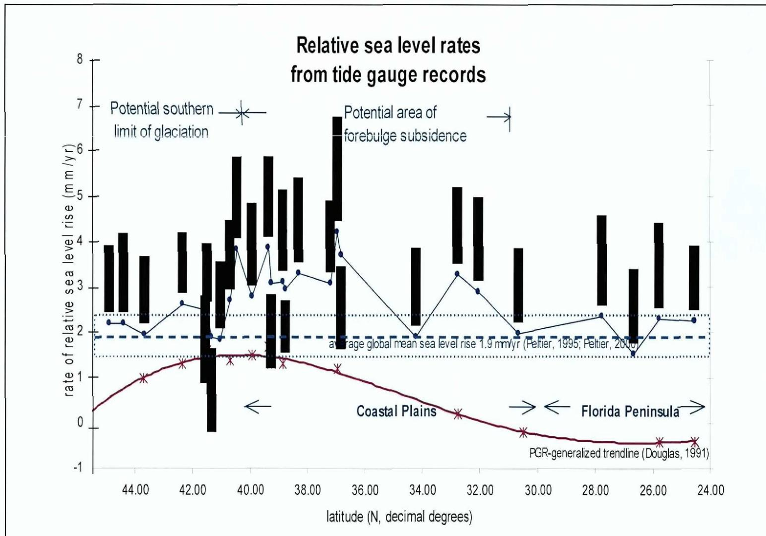
Figure 3.2: Relative rates of sea level rise along the Atlantic Coast as recorded by tide gauges. The rise in rates of subsidence (PGR) delineates the area of proglacial forebulge. (Larsen and Clark, in press)
