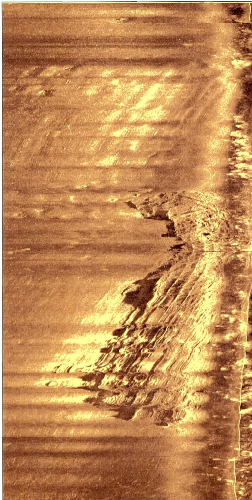
Figure 4-08. Sidescan sonar image of wreck site. Note articulated structure on north (upper) end of image.
