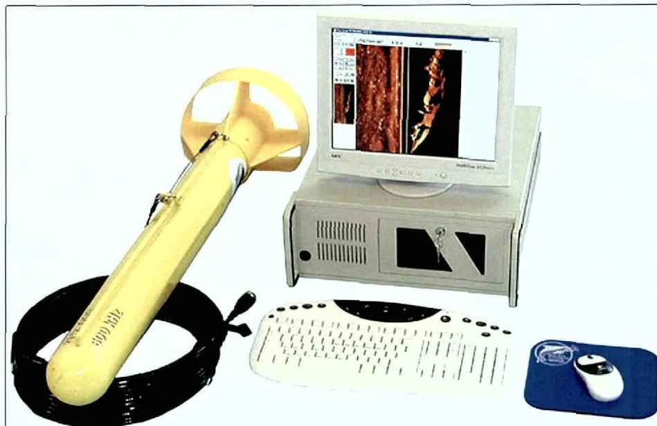
Figure 3-04. Marine Sonic Technology (MST) Sea Scan sidescan sonar system.
