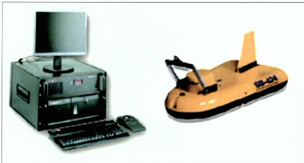
Figure 3-05. The Edgetech subbottom processor and 424 towfish used in the survey.
