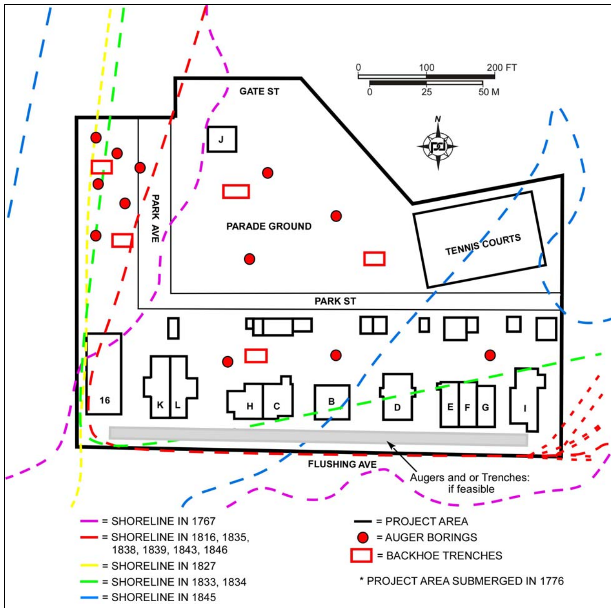
Figure 3. Suggested Phase IB geomorphological survey locations relative to historic map-documented shoreline locations at the Admiral's Row project area. Brooklyn Navy Yard, Kings County, New York. (Note: all shorelines are approximate due to the unreliable depiction of scale, location and proportions on some historic maps.)
