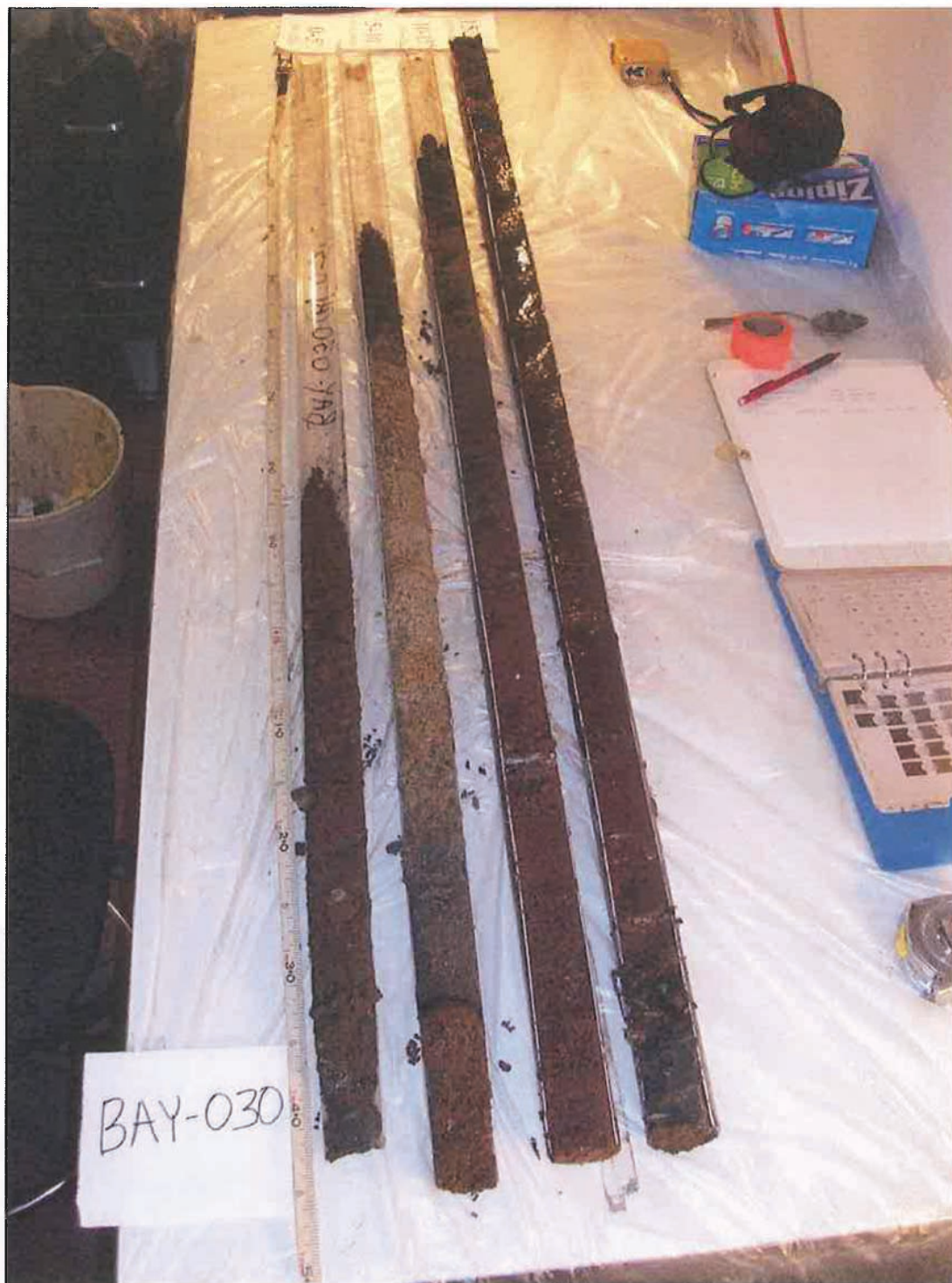
Figure 4. Split core prepared for documentation and sampling under laboratory conditions.
