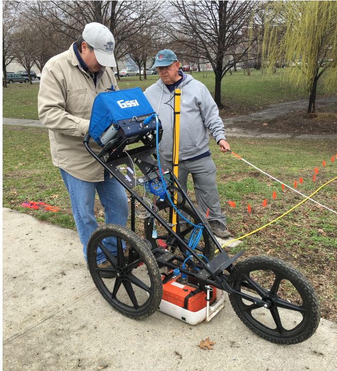
Figure 16. GSSI SIR-3000 Ground Penetrating Radar with 400 MHz antenna operated by Edwin Muñiz of the USDA.
