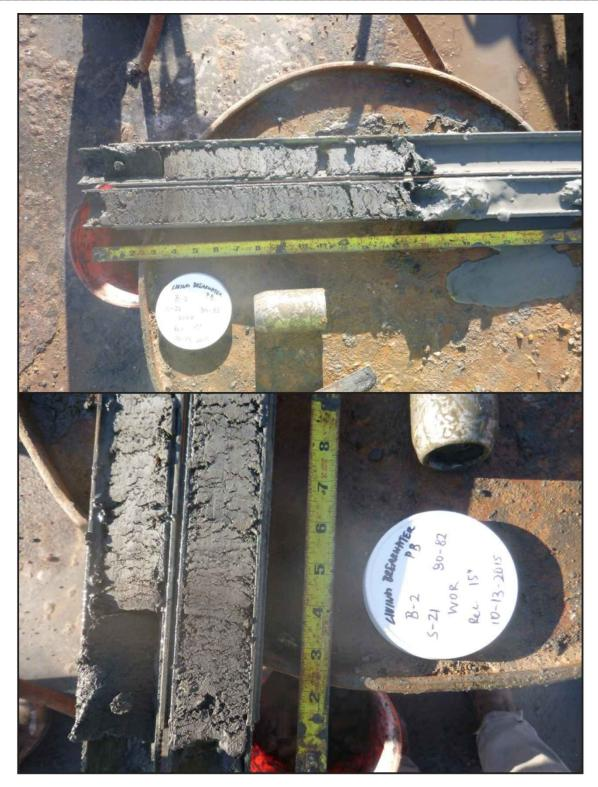
Figure 5. Photograph of bore segment 72-74 ft (79.2-81.2 ft bmsl) at bore location B-2 (top), and a close up photograph of grayish brown clay silt with botanical inclusions 80.8-81.2 ft bmsl (bottom).
