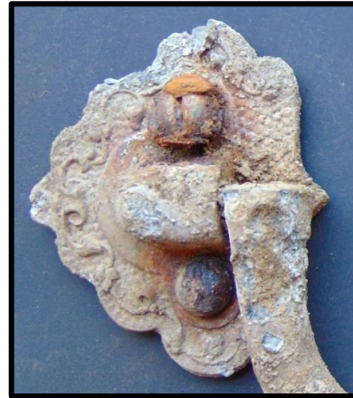
Silvered white metal swing bail coffin handles with brackets and lugs. Lugs decorated with hatching and vines (close up below) that match Russell and Erwin Manufacturing Company's handle No. 116 in their hardware catalog of 1865 (below at left).
