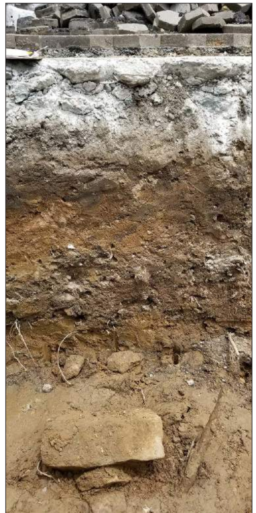
Facing north at the west end of TP1 showing the north wall profile and poured concrete pier to the left. Note that the floor of the trench is filling with water at a depth of about 6 feet bgs
