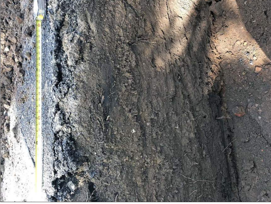
Facing south showing south wall profile of TP8, which consisted of clean sandy fills 24
