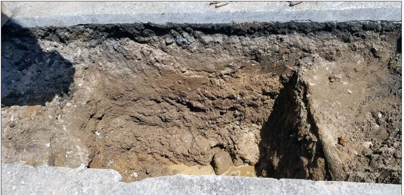
Facing north showing north wall of TP4. Note iron utility line along right side of trench, shallow, thick concrete pad on the left side of photo, mixed sandy fills, and water accumulating on trench floor at a depth of about 6 feet bgs
