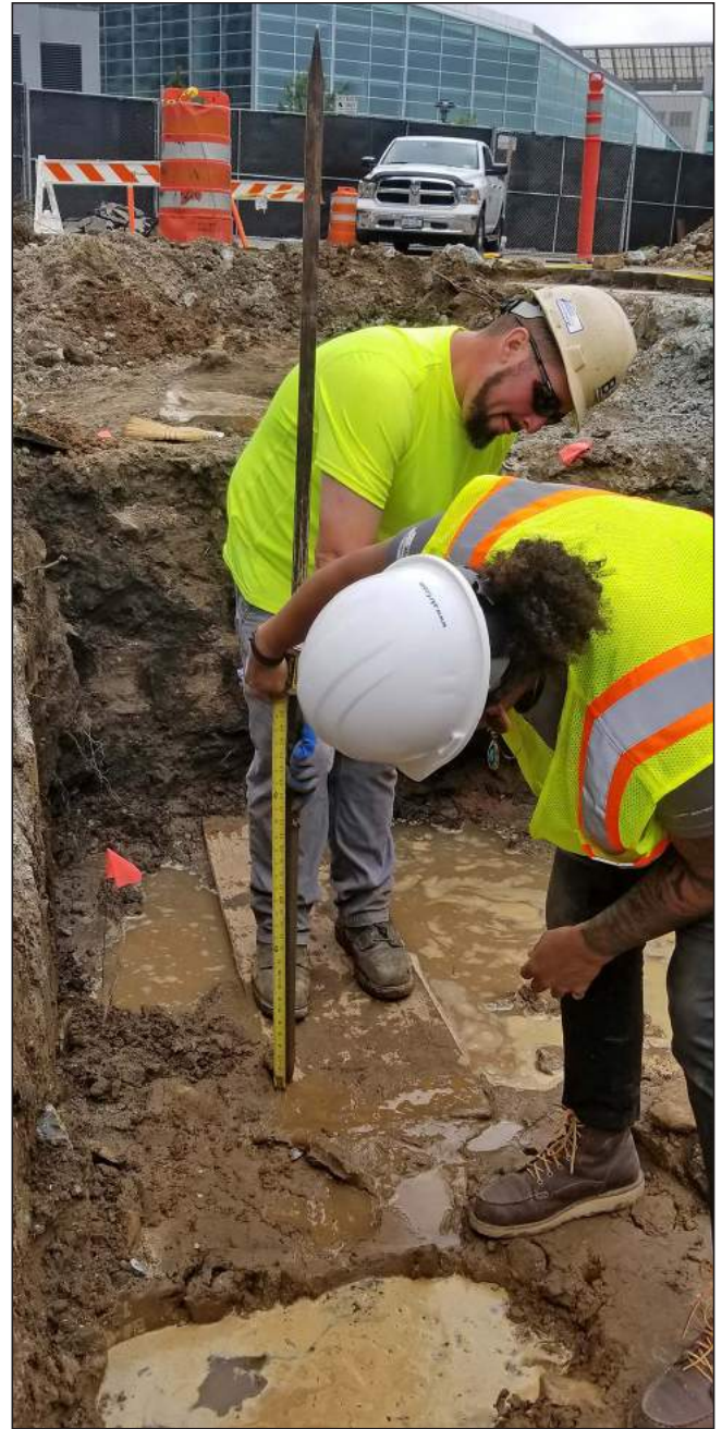
Archaeologists using a 5-foot-long pry bar to probe into the floor of TP1 to determine the depth of a rock obstruction within the water-saturated clayey soils
