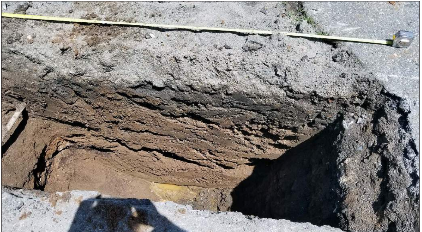
Facing north showing north wall profile of TP6. Note utility line to the left, clean sandy fills, and water accumulating on trench floor at a depth of about 6.5 feet bgs 22
