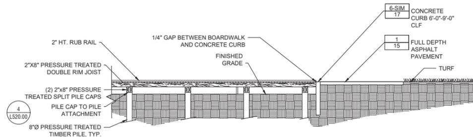
3 BOARDWALK CONNECTION AT PATH - SECTION
