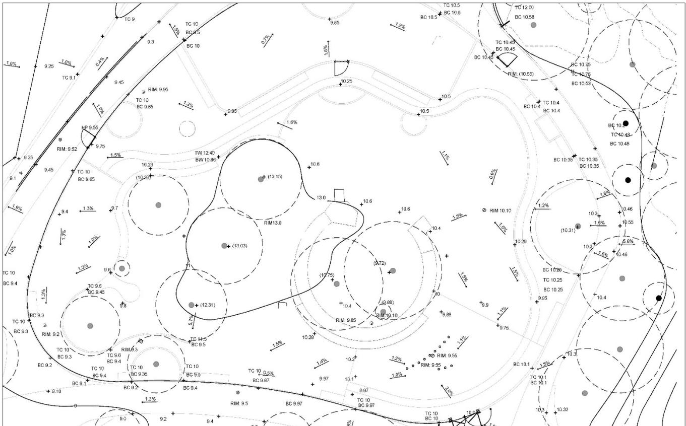
Figure 20. Comparison of existing and proposed play area. Details from topographic plan and Playground Grading Plan Enlargement, Plan Sheet L408.
