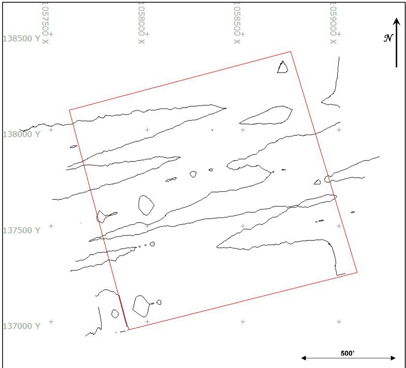
Figure 15: Magnetic Contours at 10 nT (gamma) Intervals at Offshore Borrow Area B West
