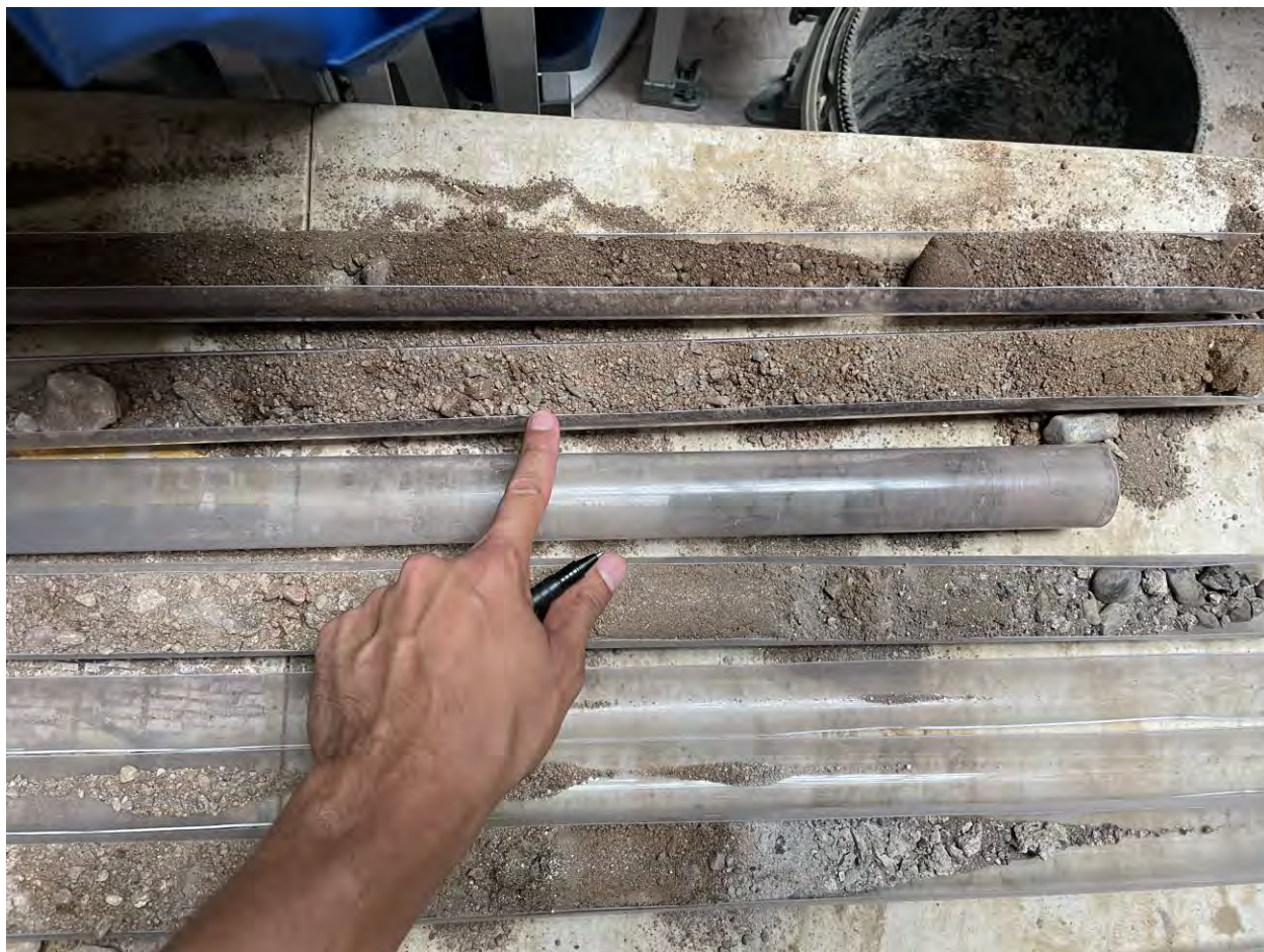
Soil from SB-1. The upper strata are on the bottom and the lower strata are on the top.
