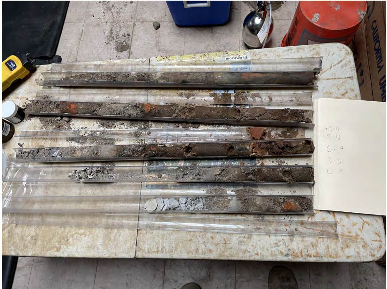
Soil from SB-3. The upper strata are on the bottom and the lower strata are on the top. Note the brick inclusions.
