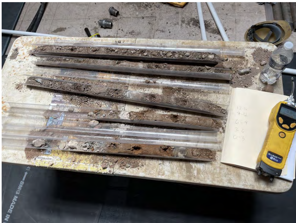
Soil from SB-2. The upper strata are on the bottom and the lower strata are on the top.
