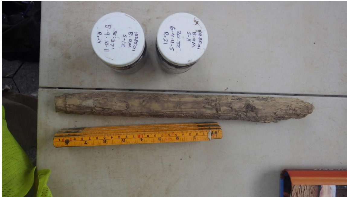
Photograph 13. Wood Timber Fragment Recovered from B12M
