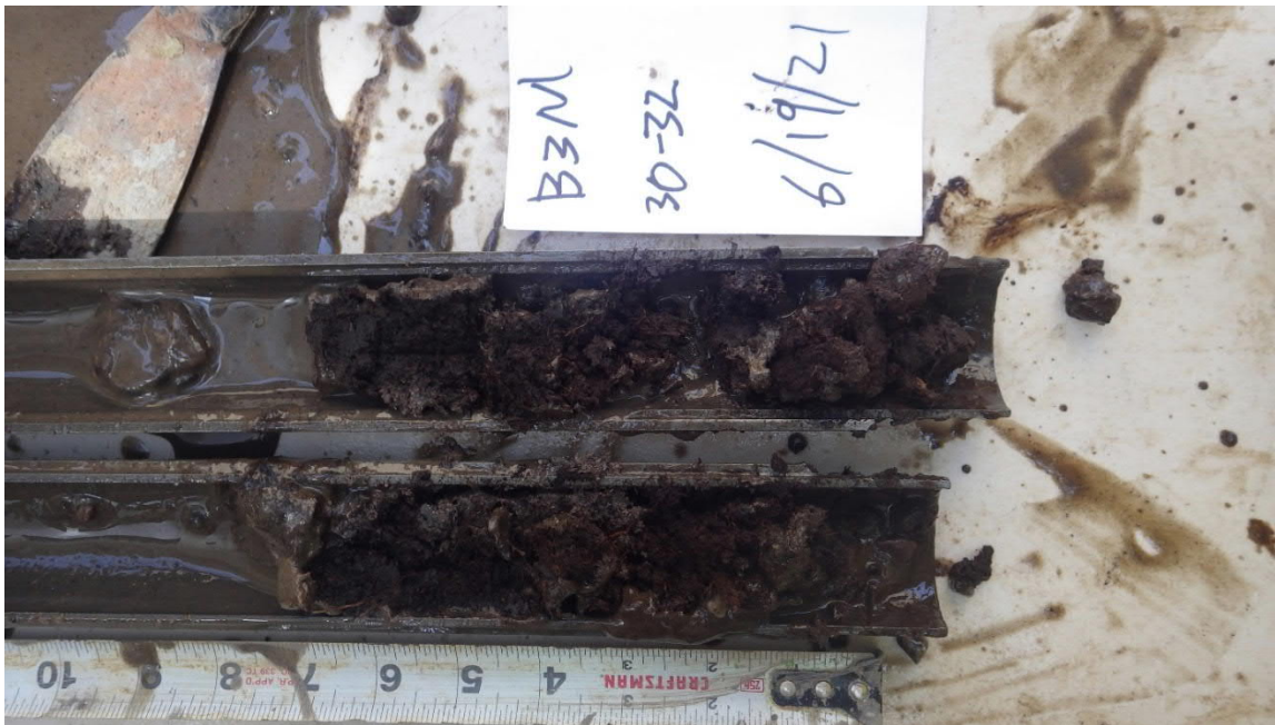
Photograph 12. Peat in B3M from 30 to 32 Feet
